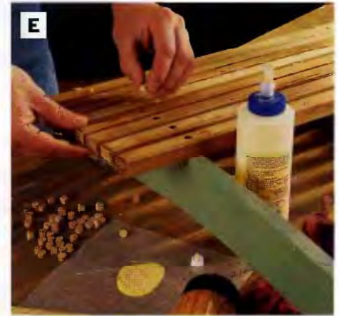
PHOTO E: Cover exposed screw heads on the slats and crossbars with oak plugs. Glue and insert the plugs, trim them and sand smooth.
