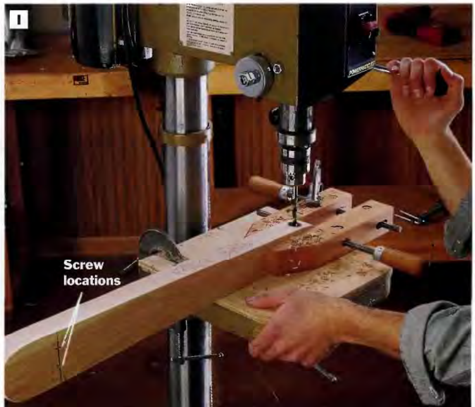
PHOTO I: Use a drill press with a Forstner or brad-point bit to drill counterbored guide holes in edges of the arms for the eyebolts.
