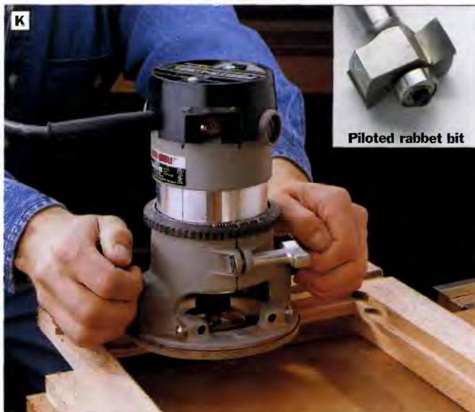
PHOTO K: Use a \frac{3}{8} -in. piloted rabbet bit (See inset photo) to cut rabbets on the insides of both side frames and the door frame. The rabbets create recesses for the glass panels. Make several passes of increasing depth with the router, until you reach the final depth ( \frac{1}{2} in.). Then square the rabbet corners with a chisel.
