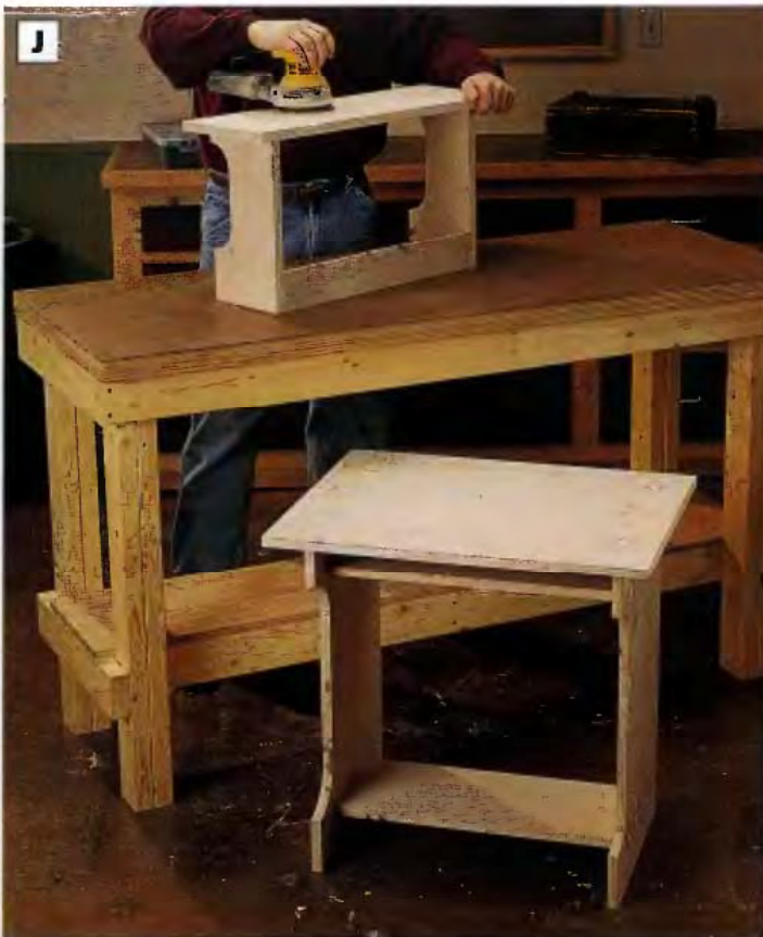
PHOTO J: Once you've filled all the screwholes and any voids in the plywood, sand the bench and desk before you prime and paint. A random-orbit sander and 150-grit sandpaper will make this a quick task.
