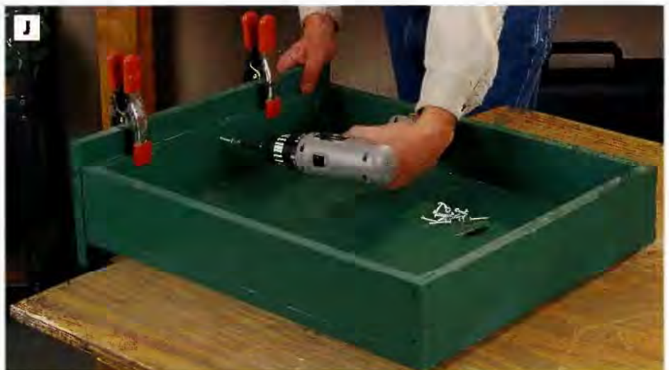
PHOTO J: Clamp the drawer face to the front of the drawer box so the ends of the drawer face are flush with the drawer sides. The face should overhang the top and bottom of the drawer by 1\frac{1}{2} in. Fasten the drawer face with 1\frac{1}{4} -in. deck screws, driven from inside the drawer.
