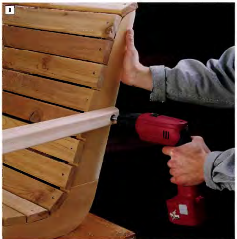
PHOTO J: Extend the 7/16-in. eyebolt guide holes in the arms through the back supports, then attach the eyebolts with washers and nuts.
