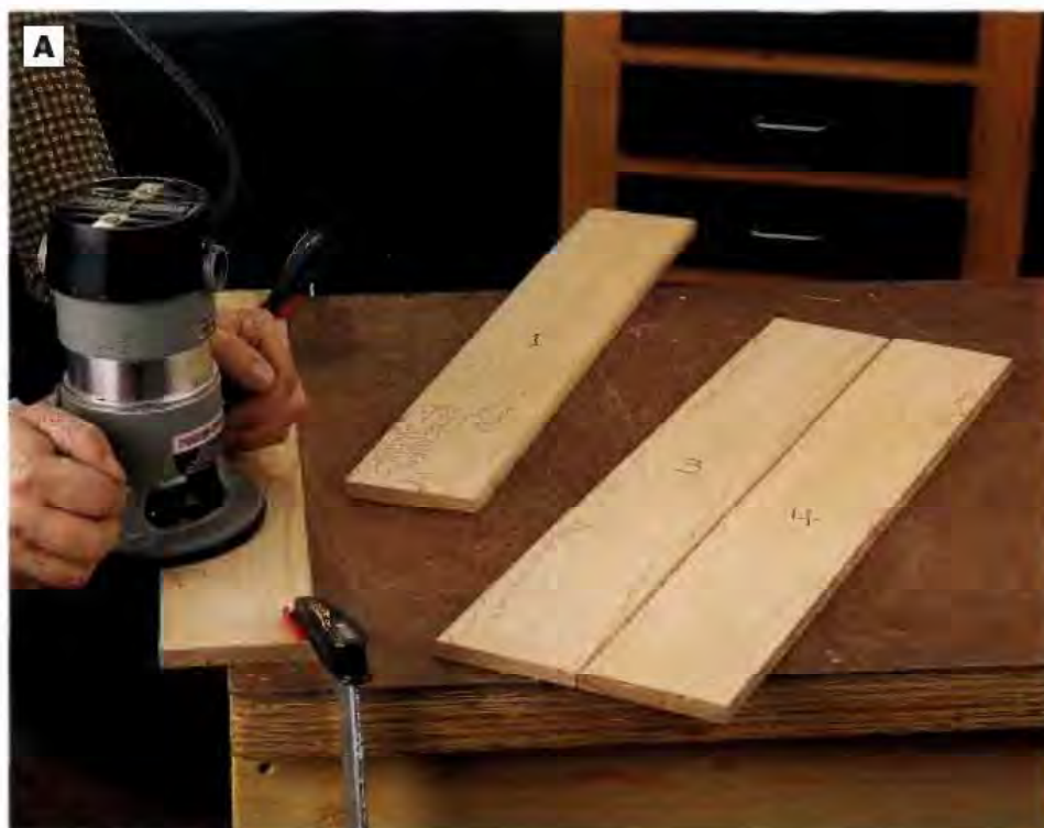
PHOTO A: Rout chamfers along the mating edges of the back slats with a piloted chamfering bit set to a cutting depth of 1 / 8 in. It's a good idea to label the slats first so you profile only the edges that will meet once the panel is glued up.
