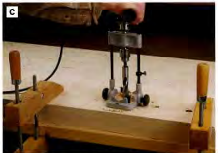
PHOTO C: Drill holes for the bench dogs at approximately 6-in. intervals, using a portable drill guide to keep the holes straight.
