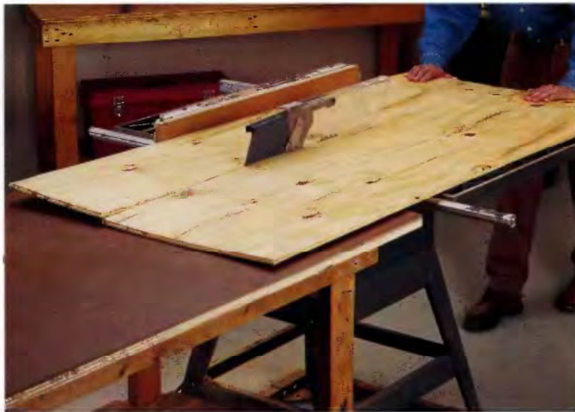
SHEET GOODS: Full sheets of plywood, particleboard and other sheet goods can be ripped effectively on a table saw if you position a sturdy table on the outfeed side of the saw, at or just below the saw table surface. But many woodworkers prefer to cut the sheets down to size with a circular saw or panel-cutting saw first.
