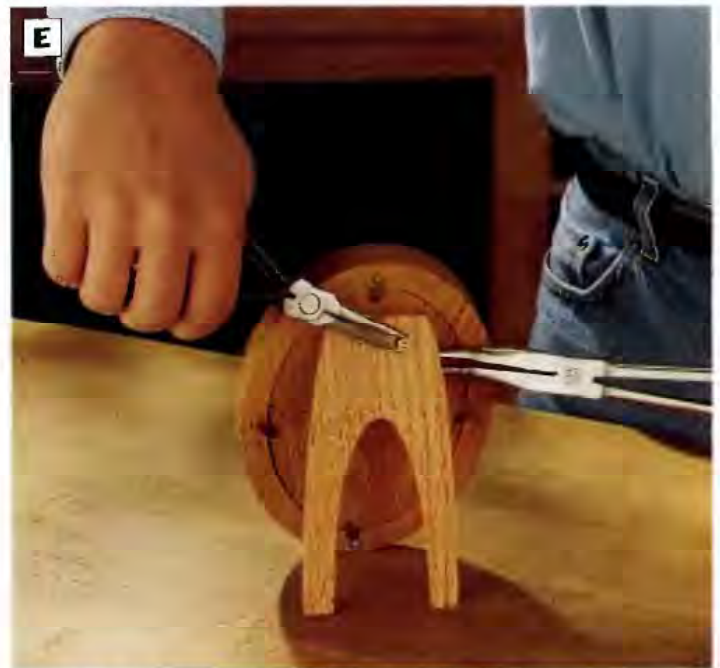
PHOTO E: After locating the hinge position, mount the hinge to the frame back with #4 x 1/4-in. brass flathead wood screws. Fasten the hinge to the stand with bolts and nuts. Arrange the bolts so you can thread the nuts on from the back of the stand. Tighten the nuts and bolts with a pair of needle-nose pliers.
