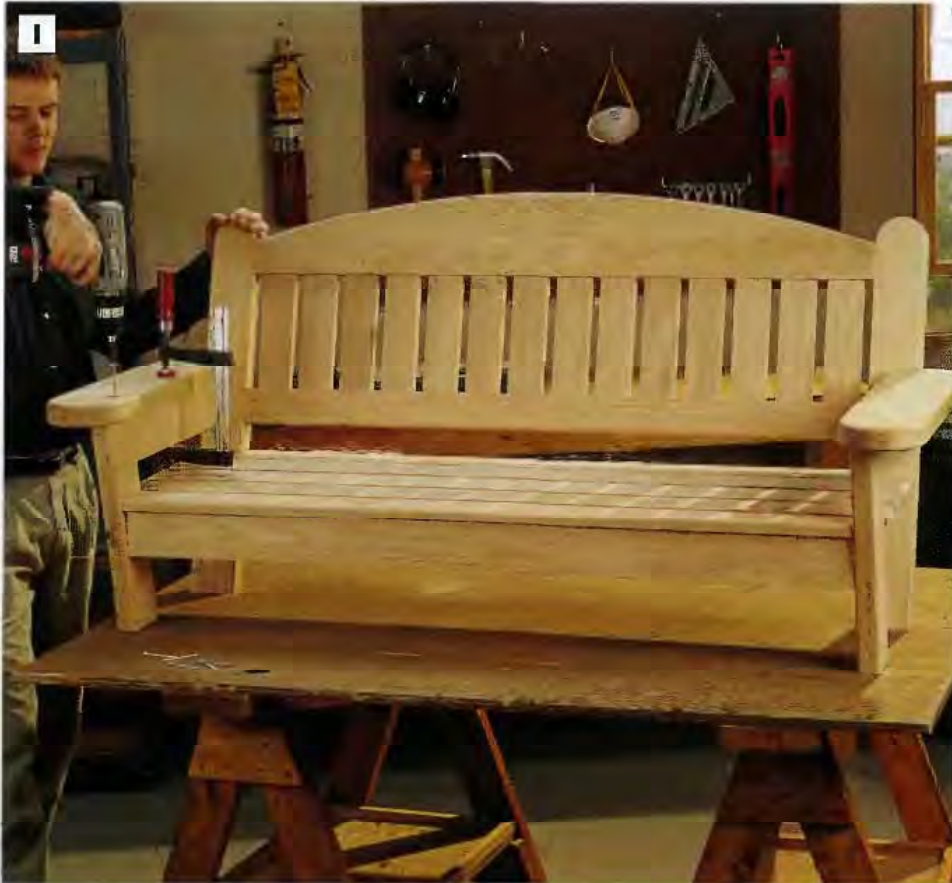
PHOTO I: Cut the arm rests to shape, ease the edges with a router and roundover bit, then clamp them on top of the arm supports. Attach the rests to the supports with countersunk screws.
