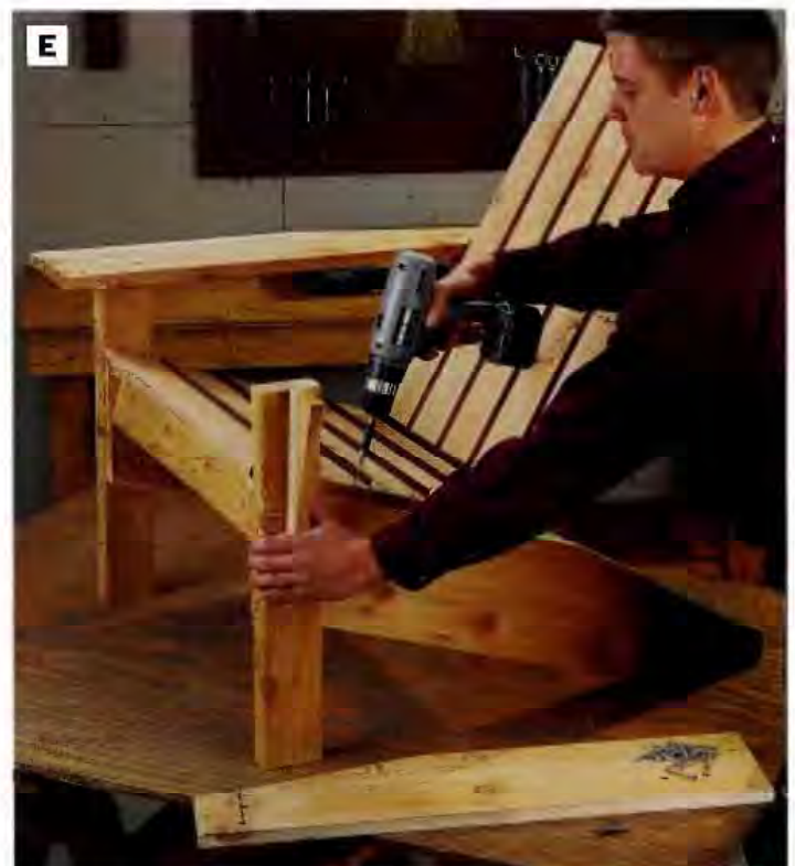
PHOTO E: Set the seat slats in place and insert ¼-in.-thick hard-board spacers between the slats. Remove one chair arm for drill clearance and fasten the seat slats to the back leg. Once the slats are attached on one side, reinstall the arm, remove the other arm and fasten the slats to the other back leg. Then reinstall the arm.
