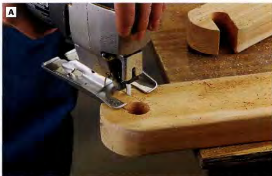
PHOTO A: Cut notches in the seat rails for back rest and foot rest dowels by boring 1-in.-dia. holes in the rails first, then cutting through the rails to the holes to form the notches. The foot rest notch (shown) is angled 45° on the seat rail, while the back rest notches are perpendicular.
