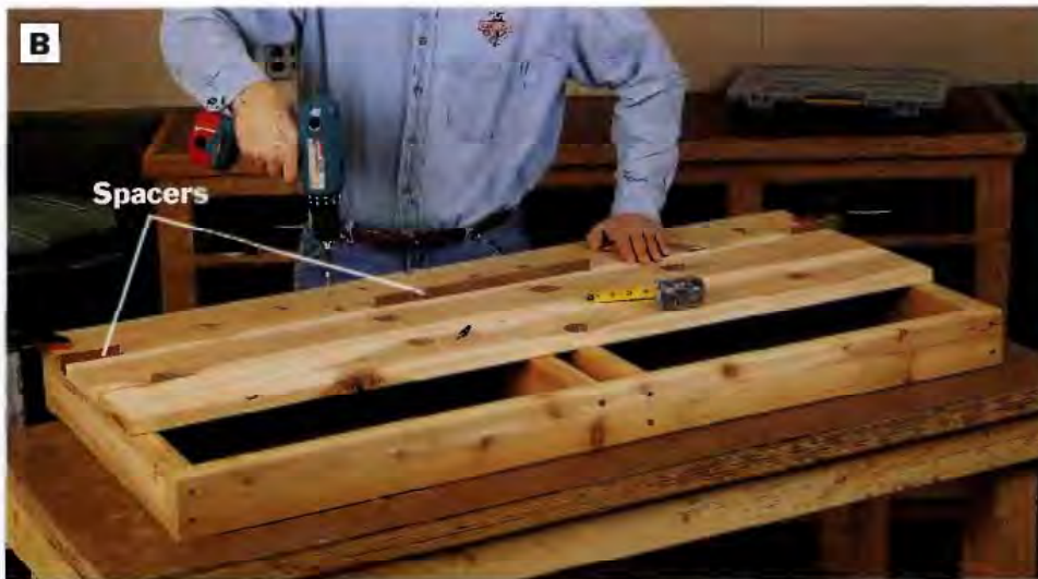
PHOTO B: Install the seat slats on the bench seat frame with screws. Position the back seat slat 7 in. from the back of the seat frame. Insert \frac{1}{4} -in. temporary spacers between the slats before screwing the slats in place.
