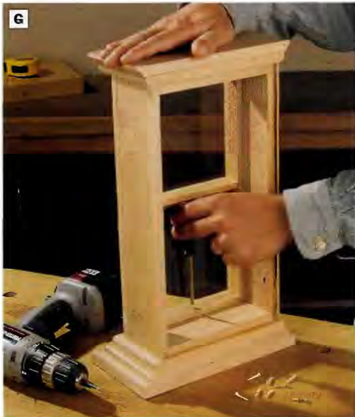
PHOTO G: Install the glass and retainer frame with a pair of brass wood screws—one through the retainer top rail and one through the bottom rail. Countersink these screws.
