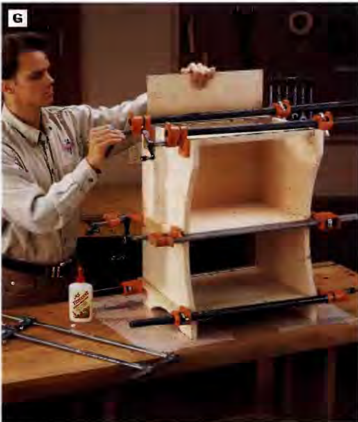
PHOTO G: After gluing and clamping the carcass together, slide the back into the side panel and bottom grooves. Loosen the clamps a bit and adjust the carcass as necessary to square it up so the top edge of the back is flush with the top edge of the rear top stretcher. Then re-tighten the clamps and nail the back to the rear top support with three or four 1-in. brads. No glue should be used with the back panel.
