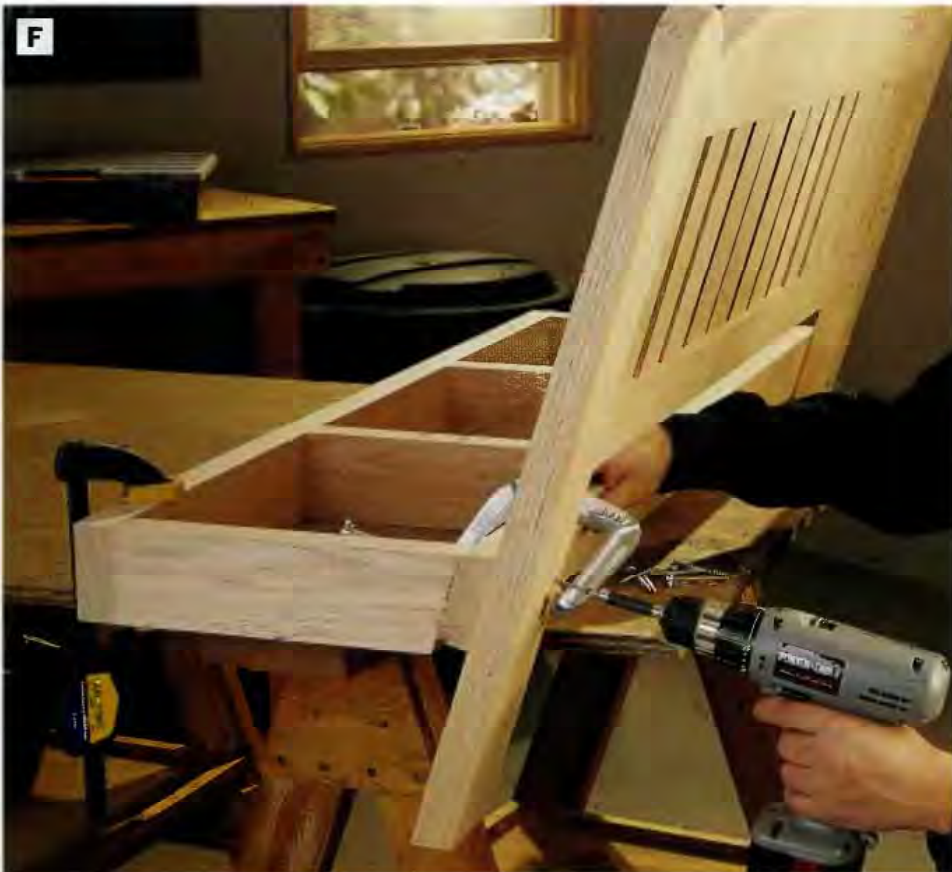
PHOTO F: Fasten the back assembly to the bench frame by driving countersunk screws through the stiles and into the back bench rail. Be sure the bottom beveled ends of the stiles are parallel with the bottom edges of the bench.
