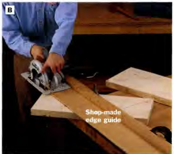
PHOTO B: Gang-cut the carcass top and bottom panels to size, then gang-cut the fixed shelves. Use an edge guide clamped to the workpiece and your workbench to ensure straight cuts.
