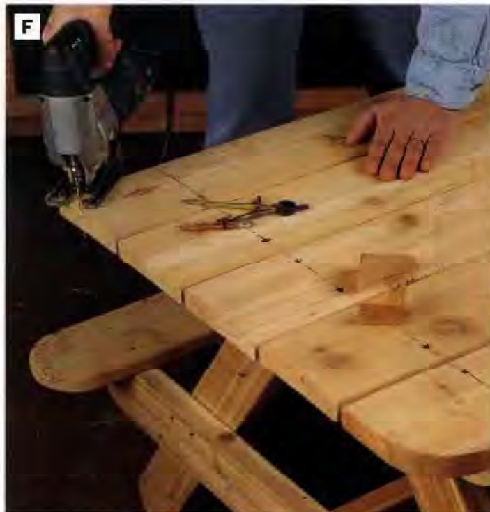
PHOTO F: Mark a 2\frac{3}{4} -in. radius on each of the four corners of the tabletop, and trim the corners with a jlg saw.
