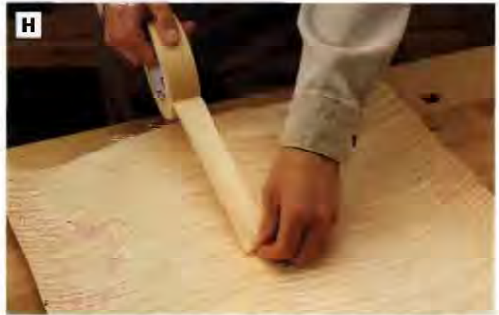
PHOTO H: Tape the jointed edges of the veneer together. Use short strips of tape to hold the joint tight. Then lay a strip down the entire length of the seam.
