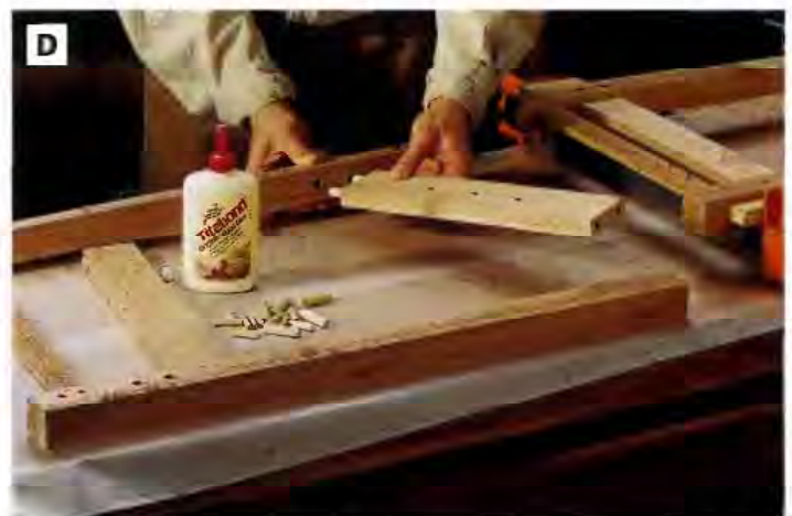
PHOTO D: Using dowel joints, glue and clamp up the legs and cross supports on a flat surface. Waxed paper protects your worksurface from glue spillage.
