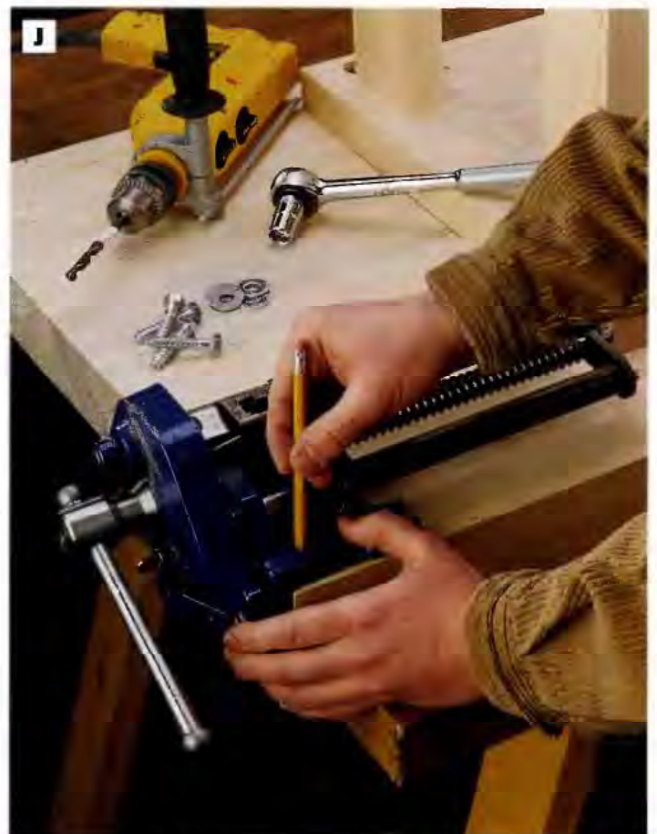
PHOTO J: Install the vise or vises according to the manufacturer's installation instructions (they may differ from model to model).
