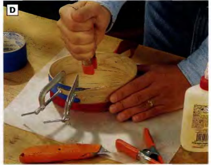
PHOTO D: Glue the side pieces to the box top and bottom. Hold the bentwood parts in position while the glue dries with strap, spring and C-clamps. Mask off the area around the fingers to protect these spots from glue squeeze-out.
