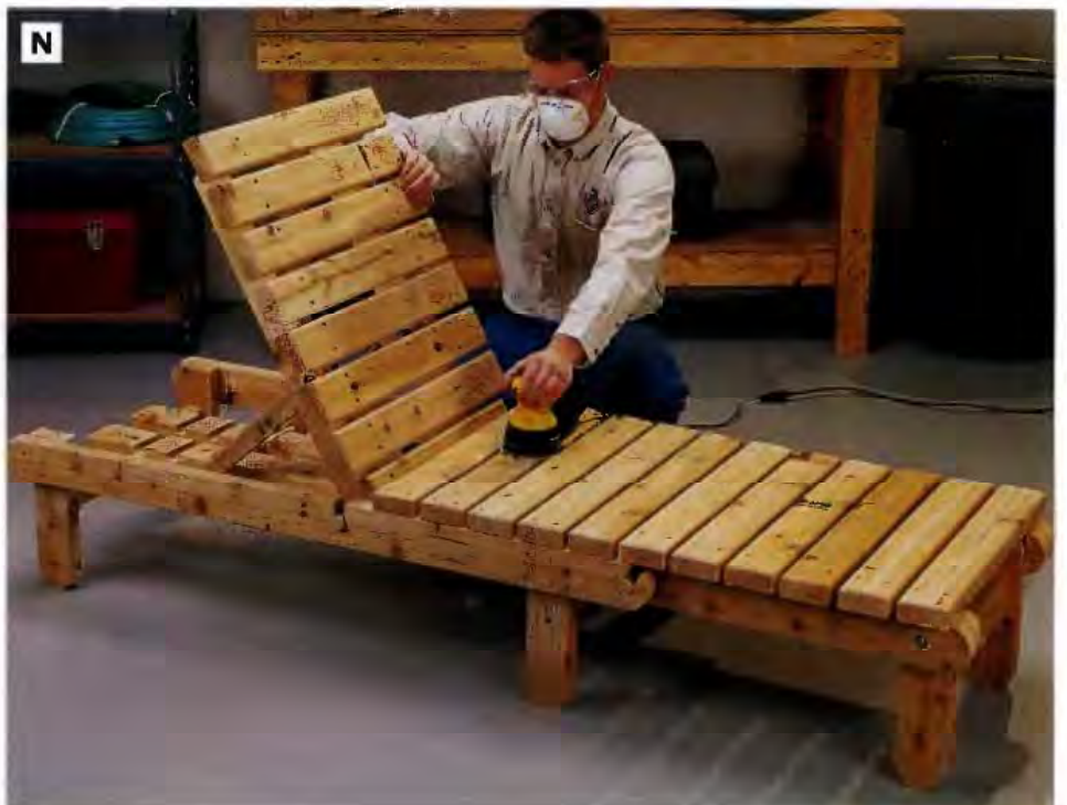
PHOTO N: Set the back and foot rests in place on the seat, and test the action of the parts. Then sand all exposed surfaces of the chair with medium-grit sandpaper. If you sand in an enclosed place, wear a particle mask. Cedar dust can be irritating to your nose and lungs.
