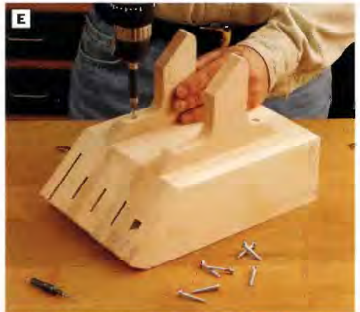
PHOTO E: Drive flathead wood screws through the feet and into the bottom of the knife block. Drill countersunk pilot holes for the screws first, to make screw installation easier and to recess the screw heads.
