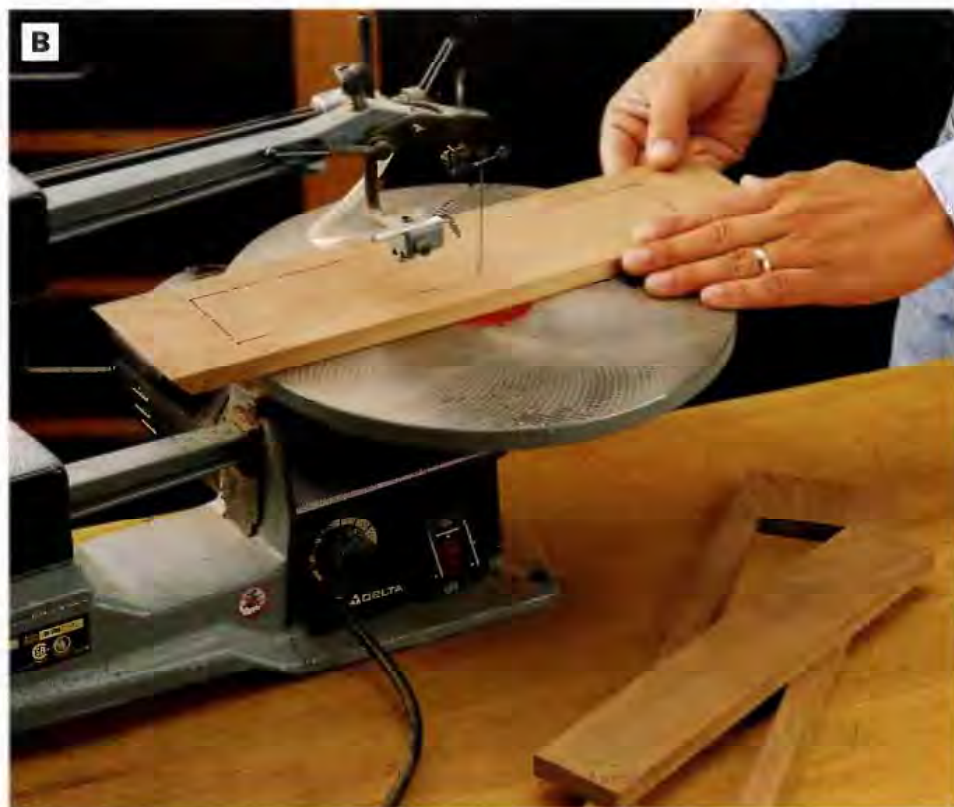
PHOTO B: After drilling starter holes at all four corners of both drawer faces, carefully cut out the faces from the front and back workpieces. The faces are cut from the front and back parts so the wood grain will match when the drawers are closed.
