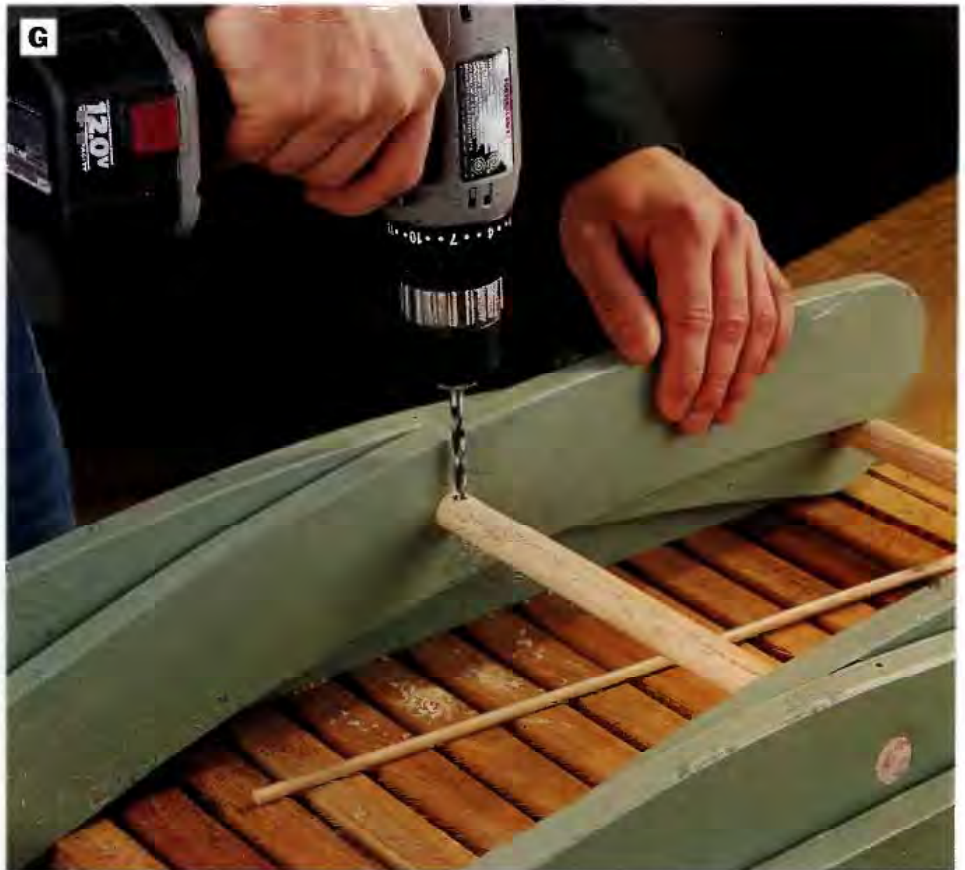
PHOTO G: Lock the inner legs in place by drilling and inserting \frac{1}{4} -in.-dia. dowels through the leg pivot dowel. Position the lock dowels to leave a slight bit of room between the legs, so they can move easily past one another without damaging the painted finish of the parts.
