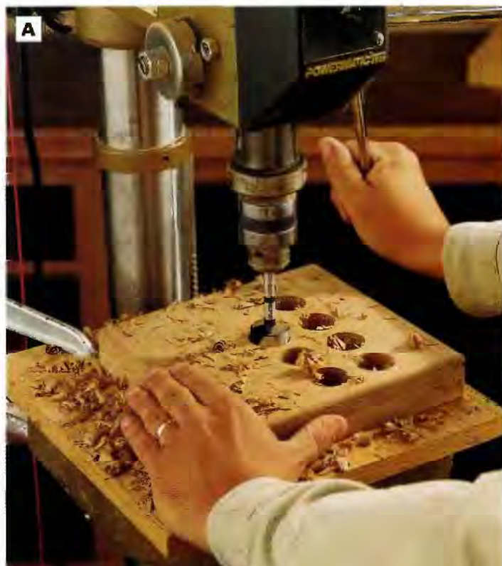
PHOTO A: (Optional) Drill three rows of 1¼-in.-dia. holes into the top face of both bases with a Forstner bit in the drill press. These holes will be filled with ballast and concealed by the base caps.
