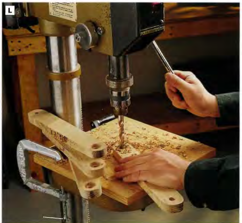
PHOTO L: Bore 5/16-in.-deep, 1-in.-dia. counterbores on both ends of the glider arms. Notice that the counterbores are on opposite faces of the arms. Then drill a 1/2-in.-dia. hole through the center of the counterbores all the way through the arms, to accommodate the pivot hinges.
