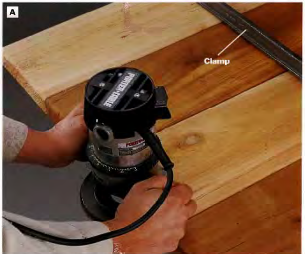
PHOTO A: Clamp the tabletop slats together and rout the ends and edges with a 1/2-in. roundover bit. Clamping the slats together will produce an even profile on the ends of the slats.
