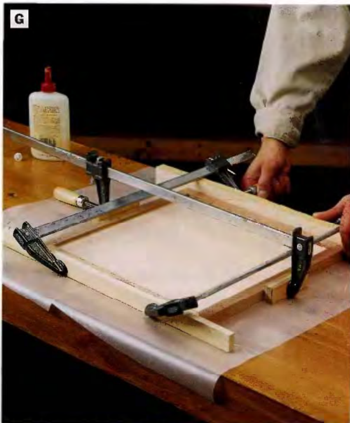
PHOTO G: Glue and clamp the tray sides to the tray bottom, aligning the mitered corners. No additional reinforcement is required.
