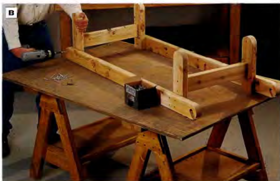
PHOTO B: Fasten the leg assemblies to the seat rails with 2½-in. galvanized deck screws. Be sure the foot rest notches on the seat rails face down on your worksurface when you fasten the legs to the rails. Check the leg assemblies with a square to be sure they are perpendicular to the rails before driving the screws.
