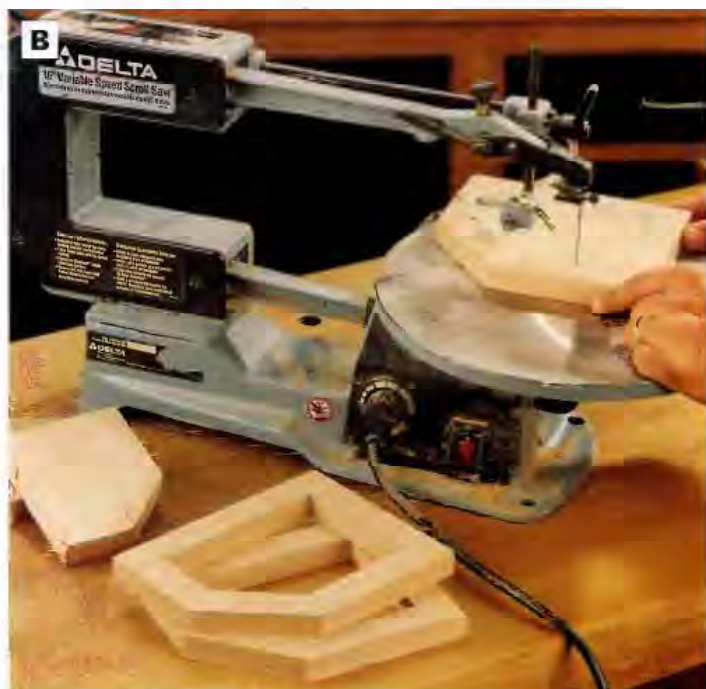
PHOTO B: Lay out and cut one frame to shape on the scroll saw, then use this first frame piece as a pattern for tracing the shapes of the other seven frames. To remove the center cutout from each frame, drill relief holes at each corner of the cutout so you can turn the workpiece on the scroll saw as you cut.
