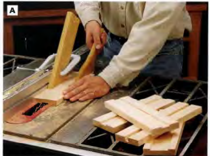
PHOTO A: Cut the knife slots into one face of the strips using a dado blade on the table saw (as shown), or on a router table with a straight bit and fence.
