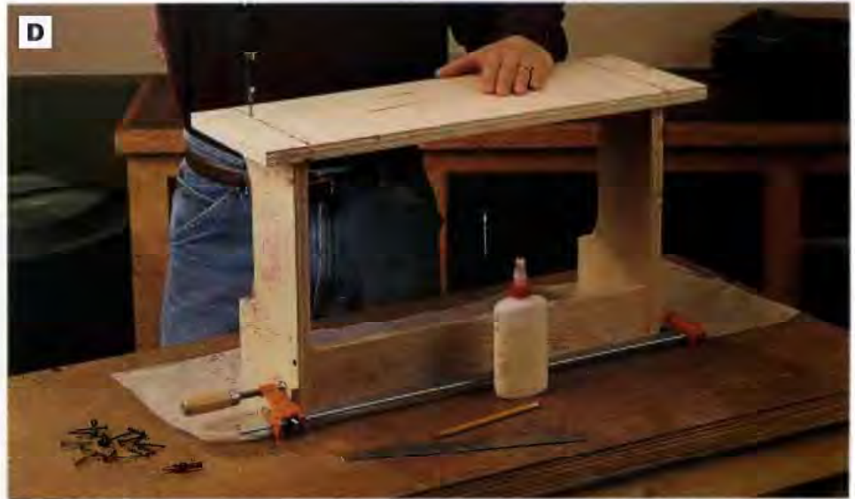
PHOTO D: After the bench stretcher is secured between the legs, fasten the bench seat with glue and countersunk 2-in. drywall screws.
