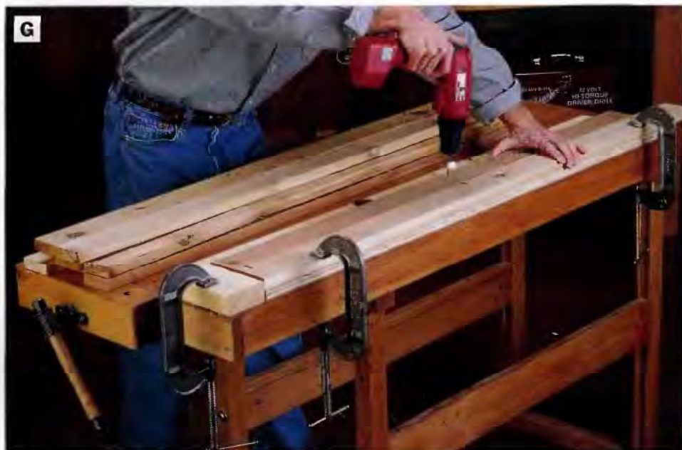
PHOTO G: Drill countersunk screw holes into the seat slats. Use a fence setup with measured guide marks for quick and consistent drilling.
