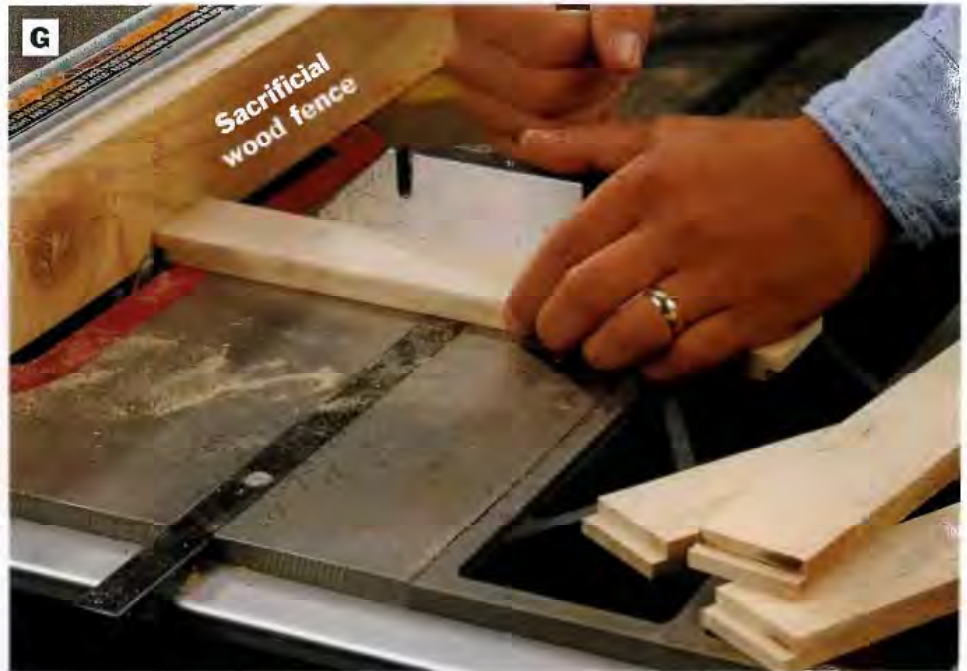
PHOTO G: Attach a sacrificial wood fence to your table saw's rip fence, and use it to establish the \frac{1}{4} \times \frac{1}{4} -in. dado blade reveal for cutting rabbets on the ends of the drawer front and back pieces. Cut the rabbets with the workpieces held against both the miter gauge and the sacrificial fence.
