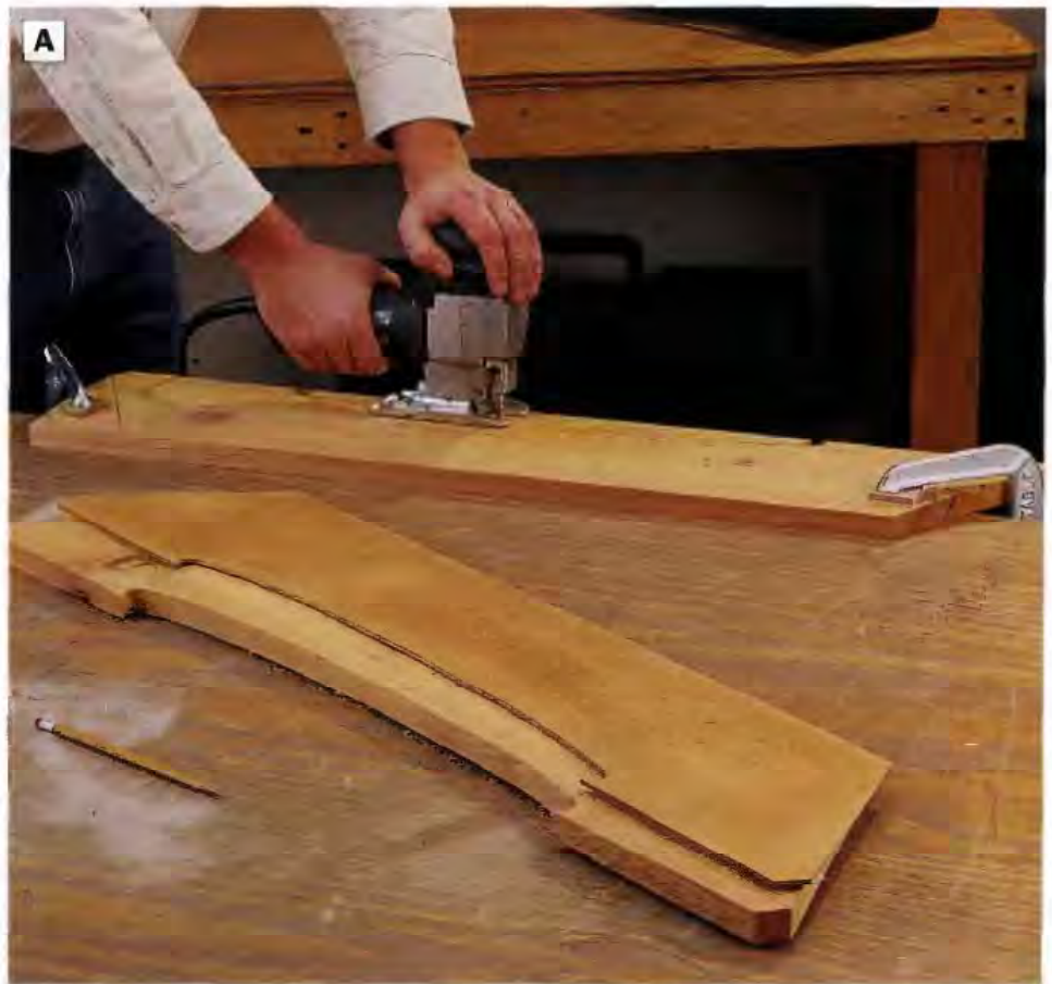
PHOTO A: Lay out and cut a template for making the sides of the railing planter, then use this template to draw the shapes on the side workpieces. Cut out the shapes with a jig saw.
