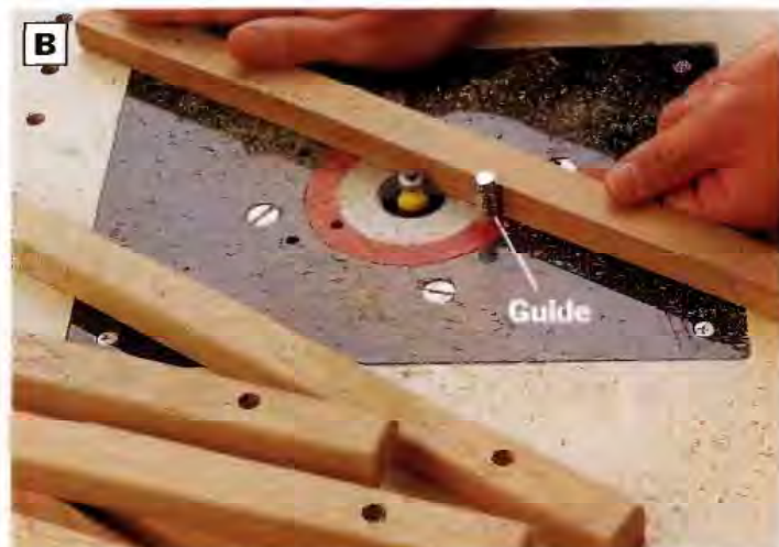
PHOTO B: Ease the edges and ends of the slats and crossbars with a \frac{1}{8} -in. roundover bit in the router table. Use a pin-style guide on the router table to help control the workpieces as you machine them.
