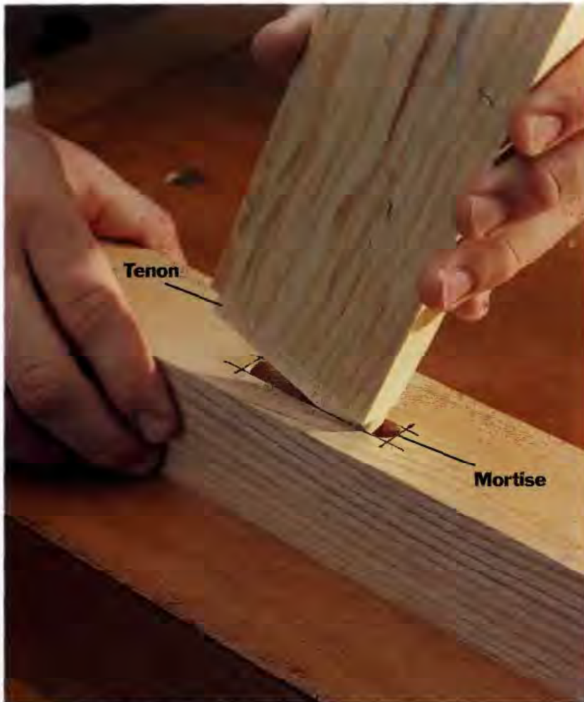
THE MORTISE-AND-TENON is one of the simplest and strongest wood joints. It's comprised of a narrow tenon carved in the end of one mating workpiece, which fits into a mortise hole in the other mating workpiece. The joint can simply be glued, or you can reinforce it with dowels or wedges.
