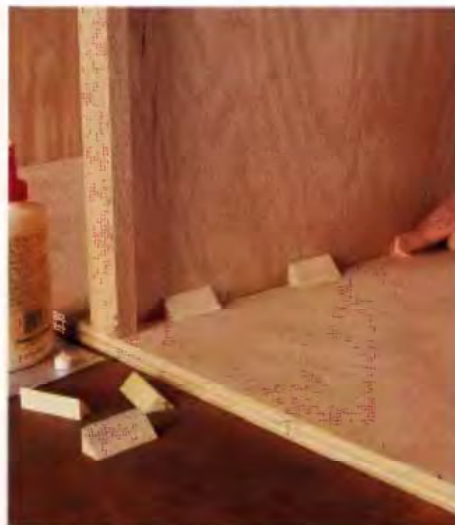
DIAGONAL GLUE BLOCKS can be glued beneath a butt joint for additional support. Use them with or without additional fasteners in the joint. The blocks are attached with glue only.
