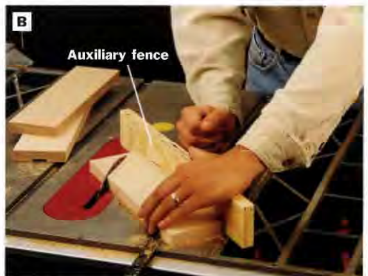
PHOTO B: Mark and trim the angled ends of the strips on the table saw with workpieces supported by the miter gauge set to a 45^\circ angle. Attach a piece of scrap to the miter gauge to serve as an auxiliary fence. Doing so provides better workpiece support and control.
