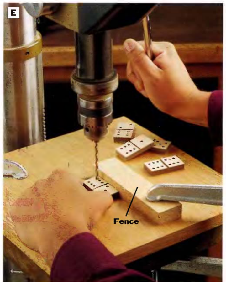
PHOTO E: Drill shallow holes through the maple veneer and just into the walnut core to create the domino dots. Set the depth stop to keep the bit from drilling too deeply. Clamp a fence to the drill press table so the rows of dots will line up lengthwise along the dominoes. Work carefully when drilling to hit your dot locations precisely.
