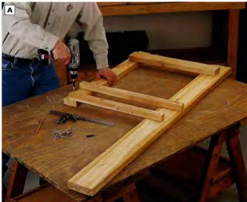
PHOTO A: Build the right assembly by attaching a drawer stretcher, drawer slide and lower stretcher between a tall leg and front leg. Fasten the parts together with 2\frac{1}{2} -in. deck screws. Use a combination square to draw layout lines for the parts and to check the joints for square.
