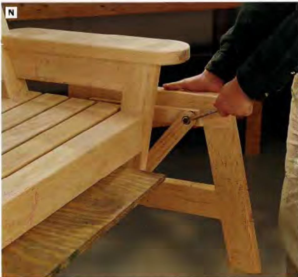
PHOTO N: Set the bench on your work surface so the glider arms hang freely. Attach the glider arms to the blocking pieces on the glider stand end assemblies with pivot hinges.
