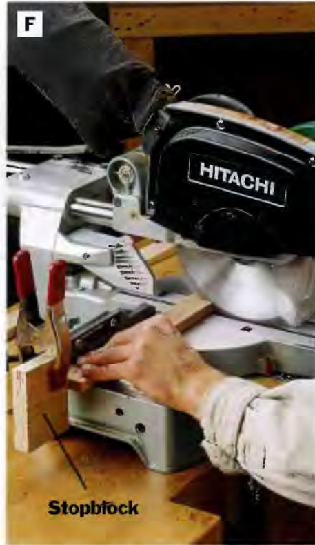
PHOTO F: Clamp a stopblock to the fence of a power miter saw, 11 in. from the edge of the blade, to make uniform cross-cuts when cutting the rails and handle pieces to length.
