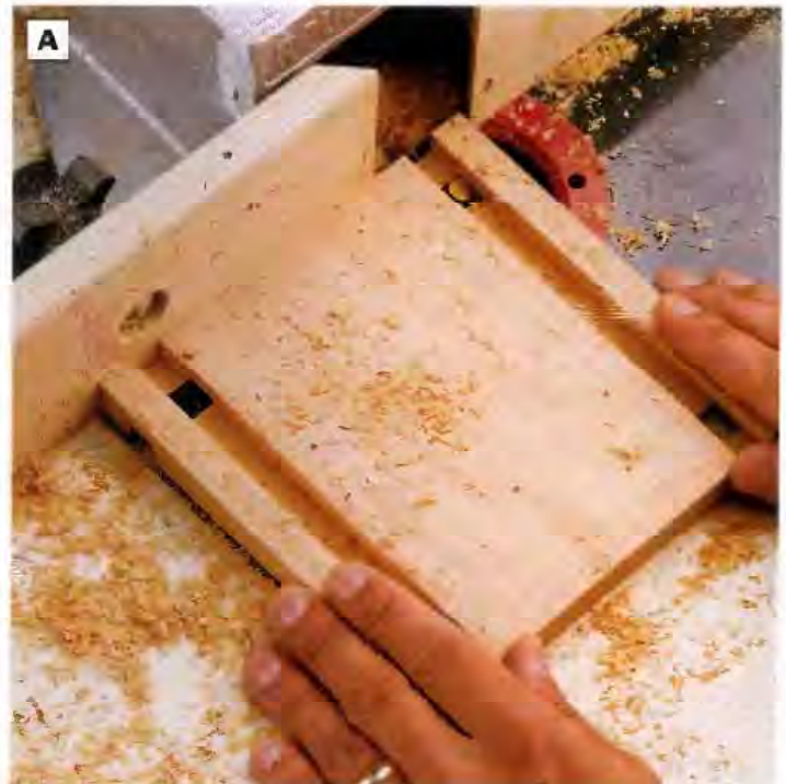
PHOTO A: Make the first series of grooves with the router fence set \frac{1}{2} in. away from a \frac{1}{2} -in. straight bit raised to \frac{3}{16} in. Cut two parallel grooves into one face, then flip the workpiece and cut two grooves in this face that are perpendicular to the grooves in the opposite face. Raise the blade to \frac{3}{8} in. and then \frac{7}{16} in., cutting progressively deeper grooves until the intersections between the grooves open up.
