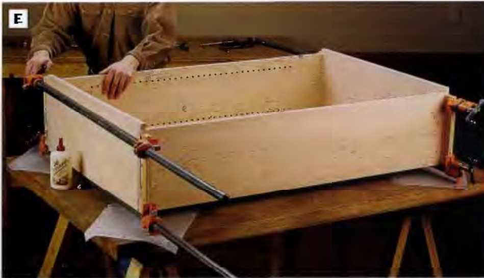
PHOTO E: Assemble the carcasses for the upper and lower cabinets. Use pairs of bar or pipe clamps and wood cauls to draw the panels together. Positioning the back panel in the back panel recess serves as a helpful reference for squaring the carcass.
