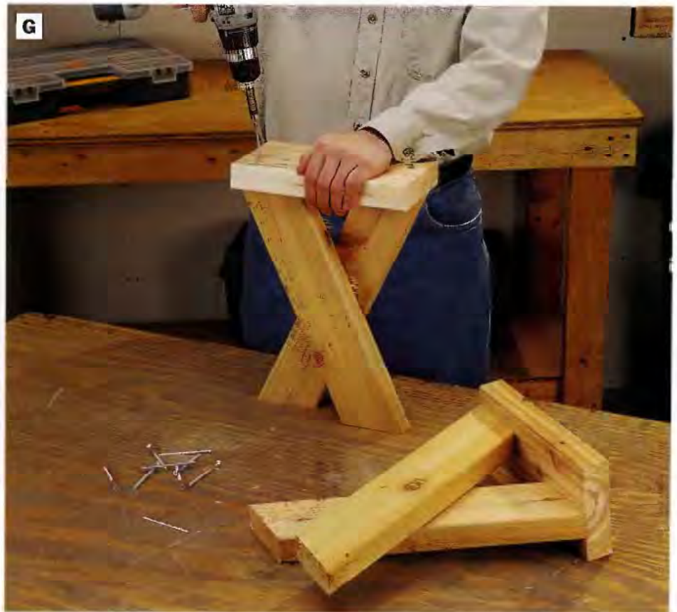
PHOTO G: Attach a bench stretcher to each pair of legs with screws. Align the top outer corners of the legs with the ends of the stretchers, and center the legs widthwise on the stretchers. NOTE: Adjust the spread of the legs on the stretchers, if necessary, so the legs will stand flat.
