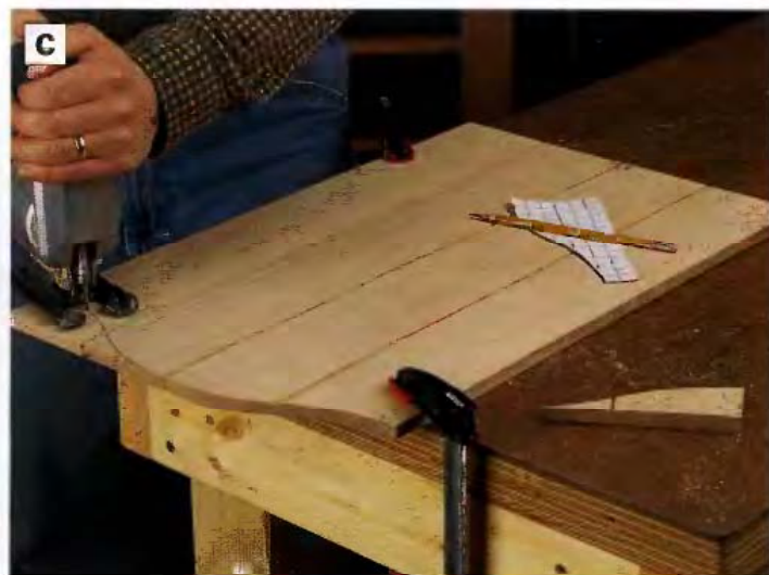
PHOTO C: Enlarge the Back Curve Layout grid pattern on page 237 to make a template for drawing the profile at the top of the back. Cut the profile to shape with a jig saw.
