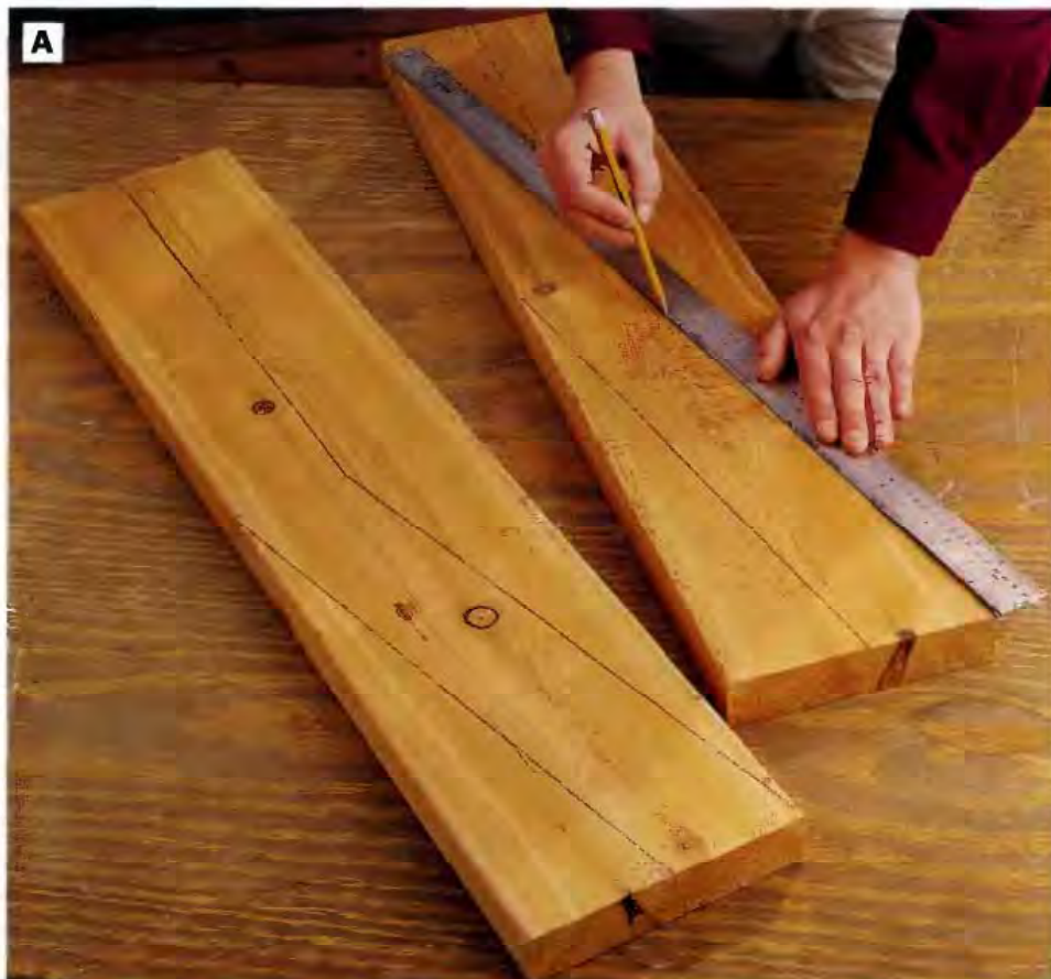
PHOTO A: Lay out and cut eight back chair legs to shape. Use the Back Legs drawing, page 389, to establish reference points for drawing the leg shapes. Connect the points with a straightedge.
