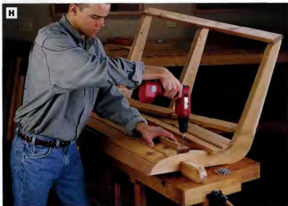
PHOTO H: Screw the slats to the back-and-seat support structures. Butt the first three slats together, then use a ¼-in.-thick spacer between the rest of the slats for consistent gaps. Keep the ends of the slats flush with the sides of the supports.
