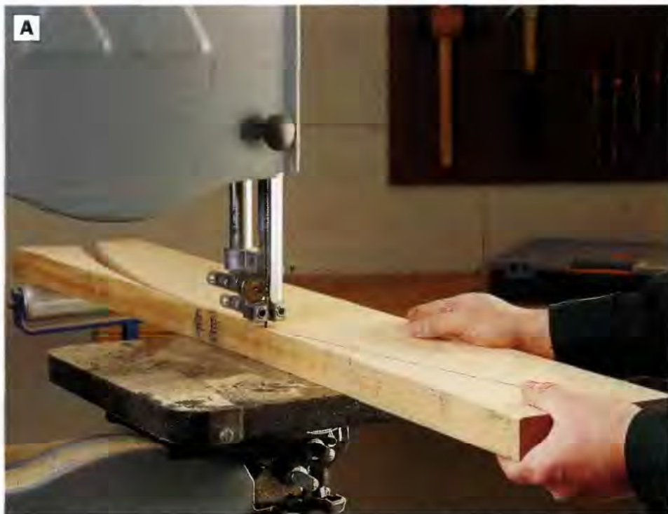
PHOTO A: Cut the profile on the upper back rail to shape on the band saw. Save the curved cut-off pieces to use as cauls when you clamp the back rails and slats together later.
