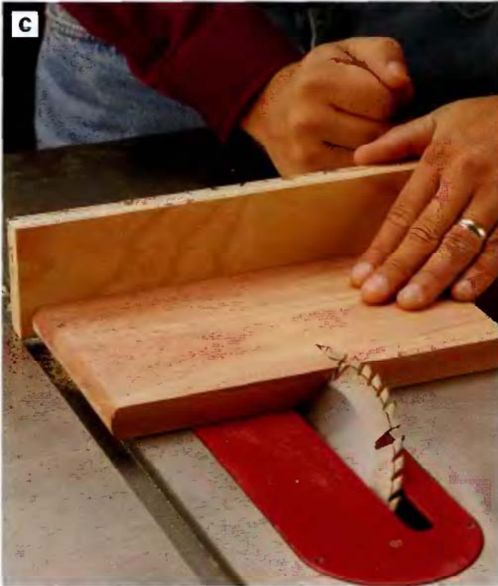
PHOTO C: Tilt the table saw blade to 45° and cut the roof blank in half to form two roof sections. Take time to set up this cut accurately. Otherwise the roof section lengths won't match. One cut both trims the parts to length and forms the roof miter joint.
