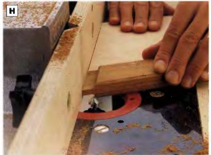
PHOTO H: Rout ⅛-in. chamfers on the ends and edges of the slats using a V-groove bit in the router table. Use an angled pushblock to guide the workpiece.
