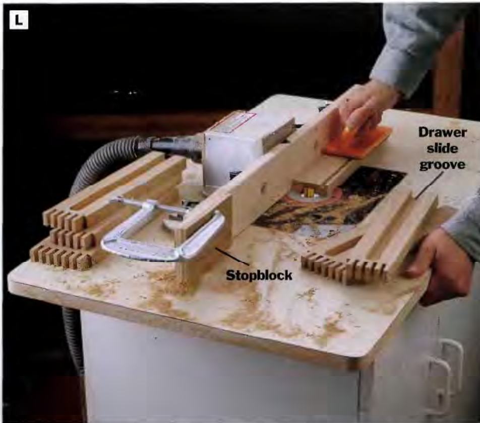
PHOTO L: After the drawer bottom grooves have been cut on the router table, rout grooves for the drawer slides. Both are stopped dados, cut in multiple passes.
