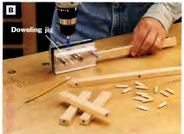
PHOTO B: Drill holes in the face frame rails and sides so you can assemble these parts with dowels. A doweling jig ensures that the holes are positioned precisely across each joint and keeps the drill bit straight in relation to the workpiece.
