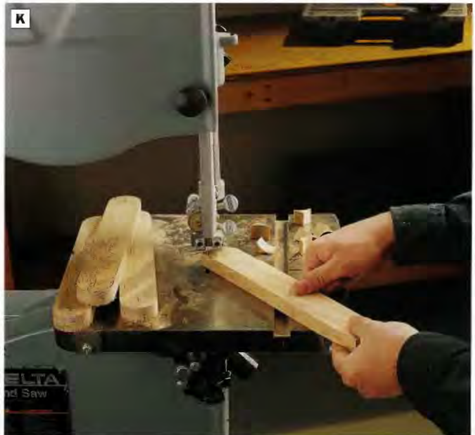
PHOTO K: Cut the four glider arms to shape on the band saw. Both ends of the arms receive 7/8-in.-radius curves. Sand the cut edges smooth and round them over with a router if you wish.
