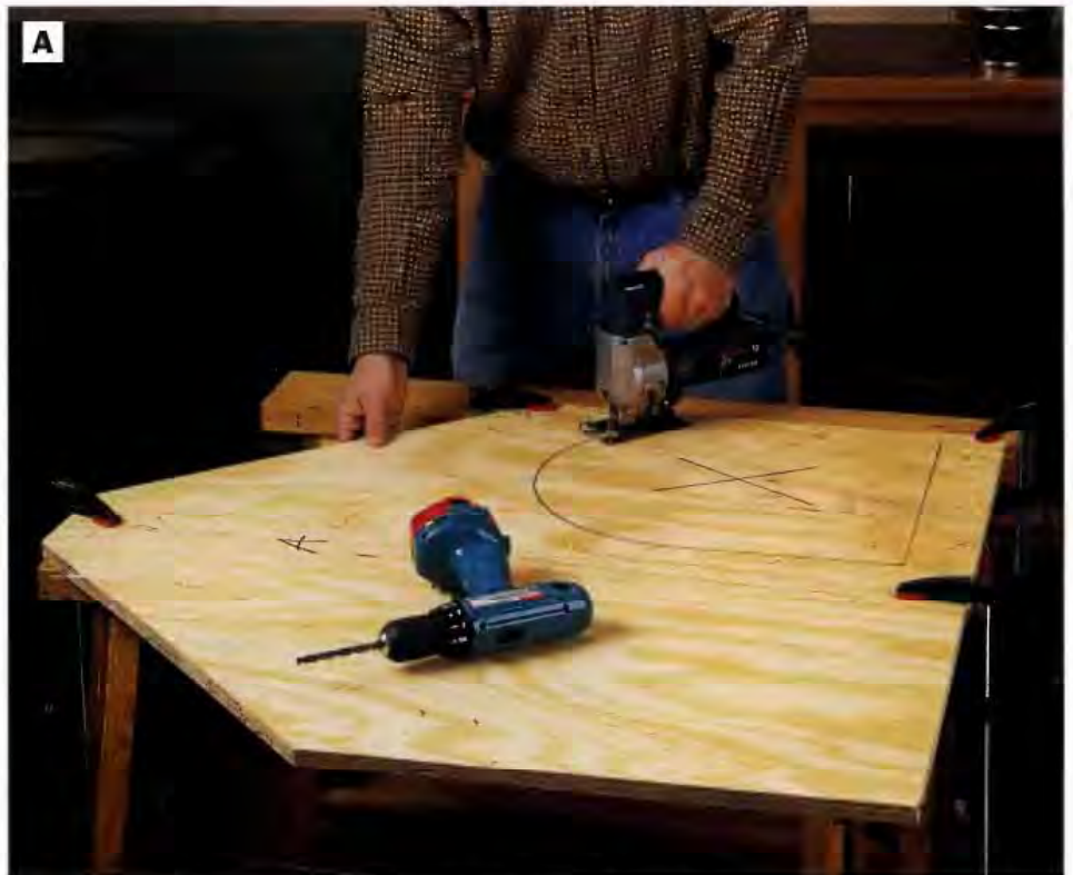
PHOTO A: Draw the arch-top door opening on the doghouse front panel, and cut out the opening with a jig saw. Drill a starter hole in the cutout area first, so you can insert the saw blade to begin the cut.
