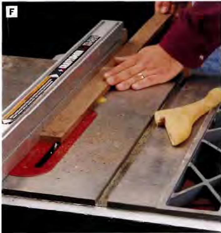
PHOTO F: Cut the ¼-in.-wide groove for the box bottom using a dado blade in the table saw. Then install a ⅛-in.-kerfed blade in the saw and cut a groove for the sliding lid along the opposite long edge of the workpiece. Cutting these grooves now allows you to work more safely with a long workpiece and ensures that the grooves will align perfectly when you assemble the box later.
