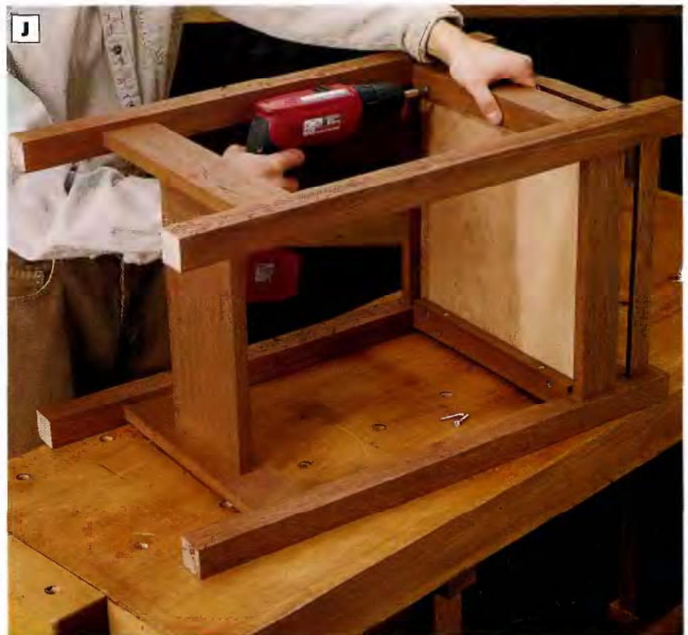
PHOTO J: Lay the plant stand on its side and attach the finished tray by driving #6 × 1-in. screws up through the countersunk screw holes in the bottoms of the tray cleats.
