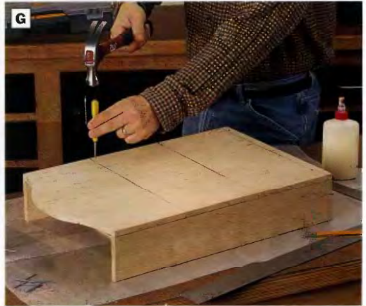
PHOTO G: The back is secured with glue and nails. Before attaching, mark a line across the back at each shelf to serve as guides for locating the fasteners. Drill pilot holes for the finish nails, and set the heads so they will not scratch the wall once the shelf unit is hung.
