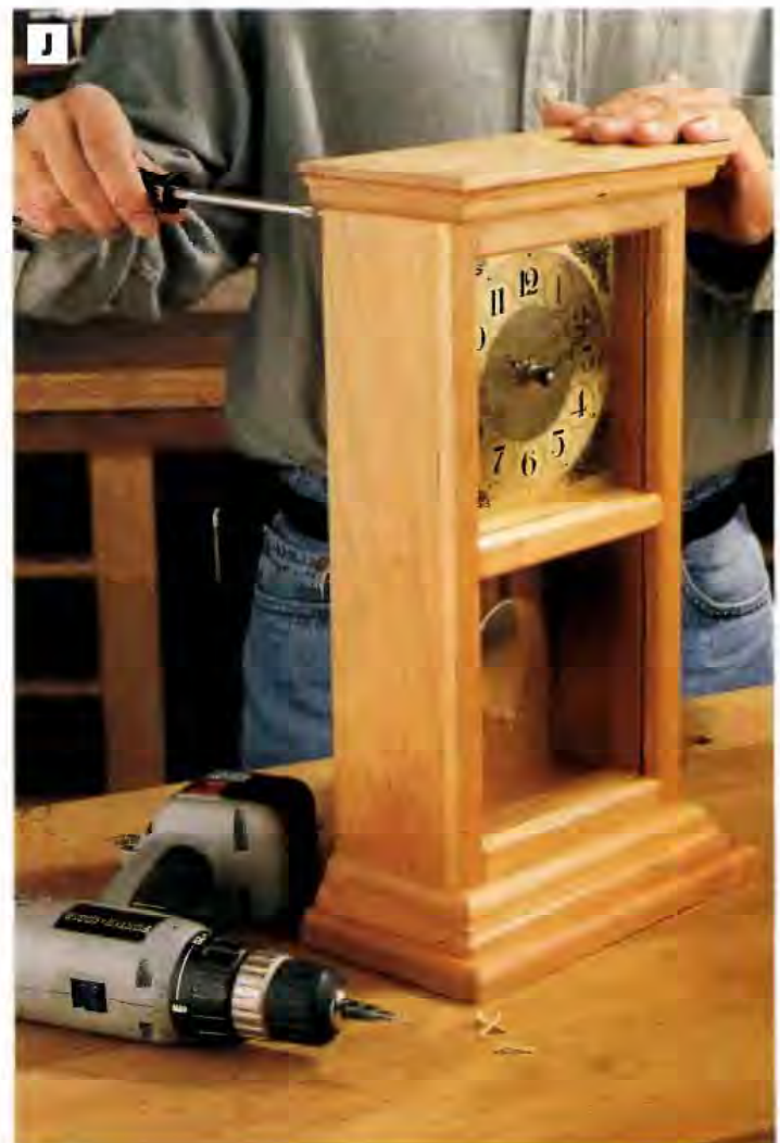
PHOTO J: Apply your finish of choice to all of the wood clock surfaces, then install the clock back with brass flathead wood screws, driven through the back and into the rabbets in the carcass back.
