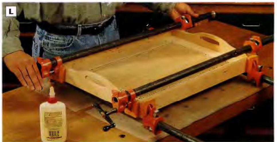
PHOTO L: Spread glue onto mating surfaces of the finger joints, slip the bottom into its grooves and clamp up the tray. Install clamps both lengthwise and widthwise to hold the finger joints closed in two directions.
