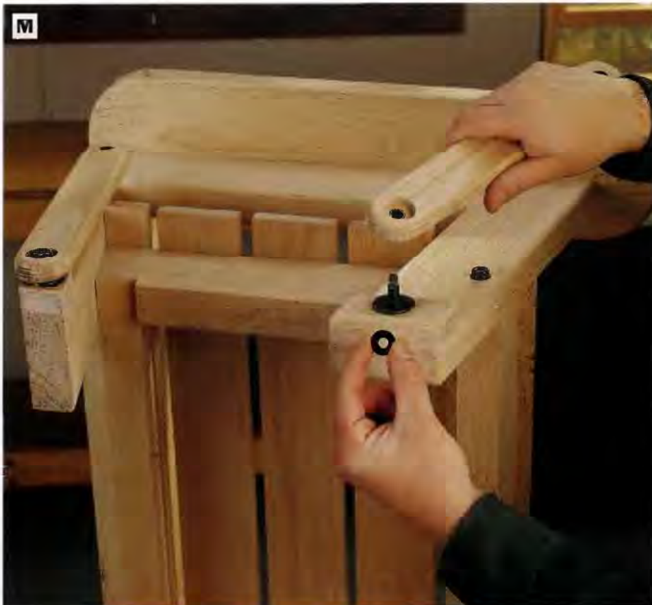
PHOTO M: Install pivot hinges to connect the glider arms to the blocking pieces on the bench. The hardware is essentially a shaft that slides inside a plastic bushing in the glider arms. The hinges press into holes in the blocking and hold the arms in place with washers and nuts.
