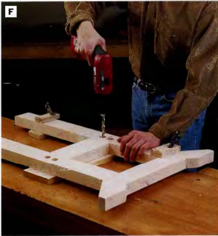
PHOTO F: Drill counterbore holes for the lag screw heads and washers, and drill clearance holes and pilot holes for the shanks of the screws.
