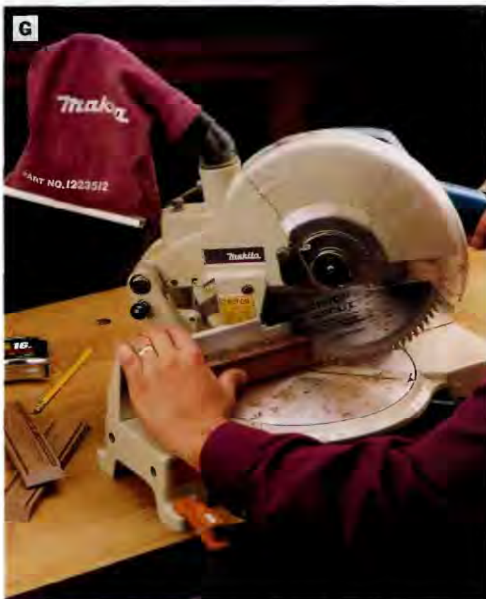
PHOTO G: Cut the box sides and ends to length. We set a power miter saw to 45° so that the parts would be both cut to length and also mitered for assembly. Accuracy is especially critical if you perform both of these operations in one step.
