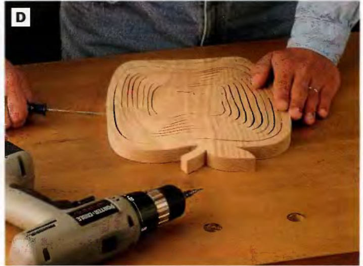
PHOTO D: Fasten the stand and the basket to the frame. Attach the basket with two \frac{3}{4} -in. brass flathead wood screws, driven into countersunk holes in the frame sides. Attach the stand to the frame with a 1-in. brass flathead wood screw, driven up from below.
