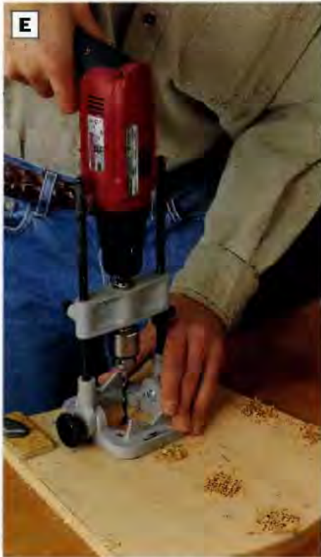
PHOTO E: Drill ½-in.-deep dowel holes at the dowel hole centers you marked on each of the two sides with the hardboard template. Use a drill guide to ensure straight holes.
