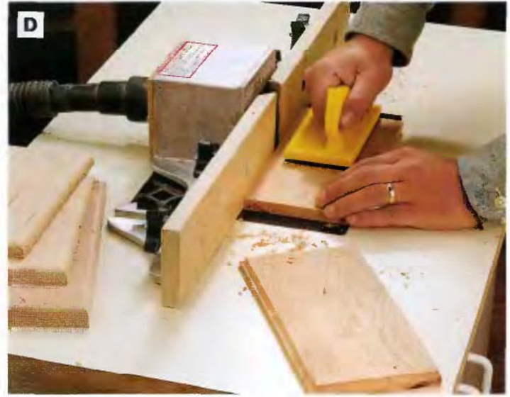
PHOTO D: Rout the roundover and cove and bead profiles into the ends and along one edge of the base and crown parts. Mill the end grain first, then rout the long grain; otherwise the bit could tear out the corners of your finished edges.
