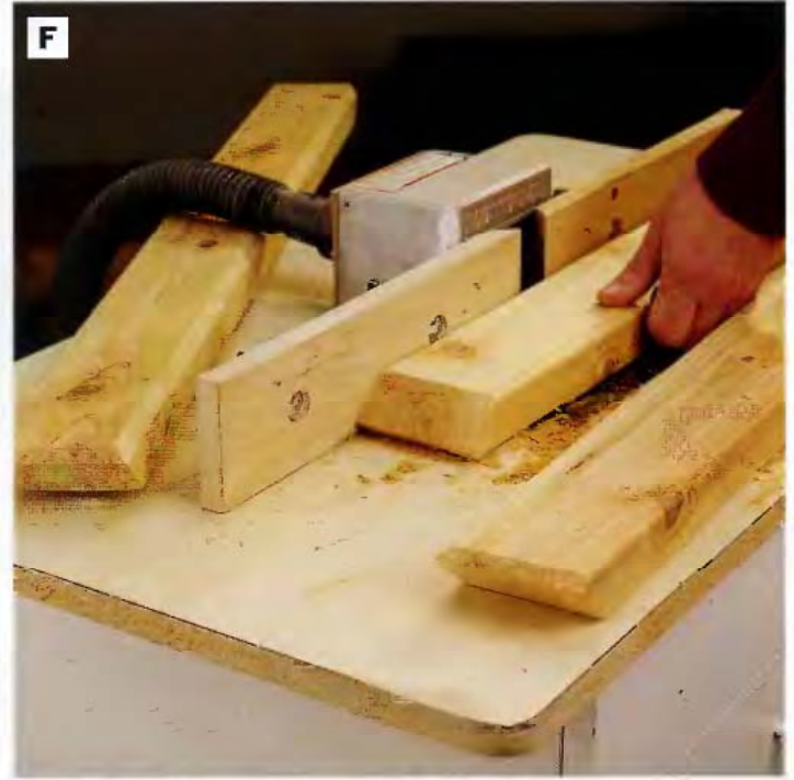
PHOTO F: The bottom edge and both ends of each apron piece are chamfered. Make these cuts at the router table, using a piloted chamfering bit set to a height of \frac{3}{8} in.
