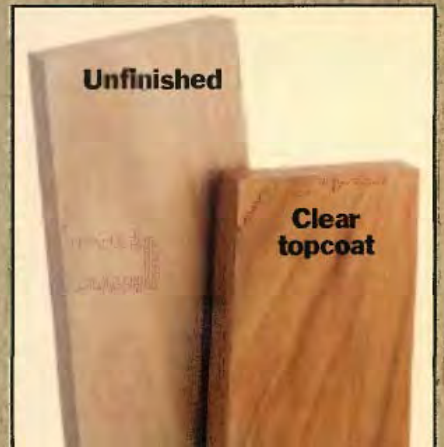
WHITE OAK is a versatile hardwood with a distinctive appearance. Used extensively in furniture-building, as well as in boat-building. It is moderate in price (quarter-sawn tends to be higher cost). Moderate workability.
