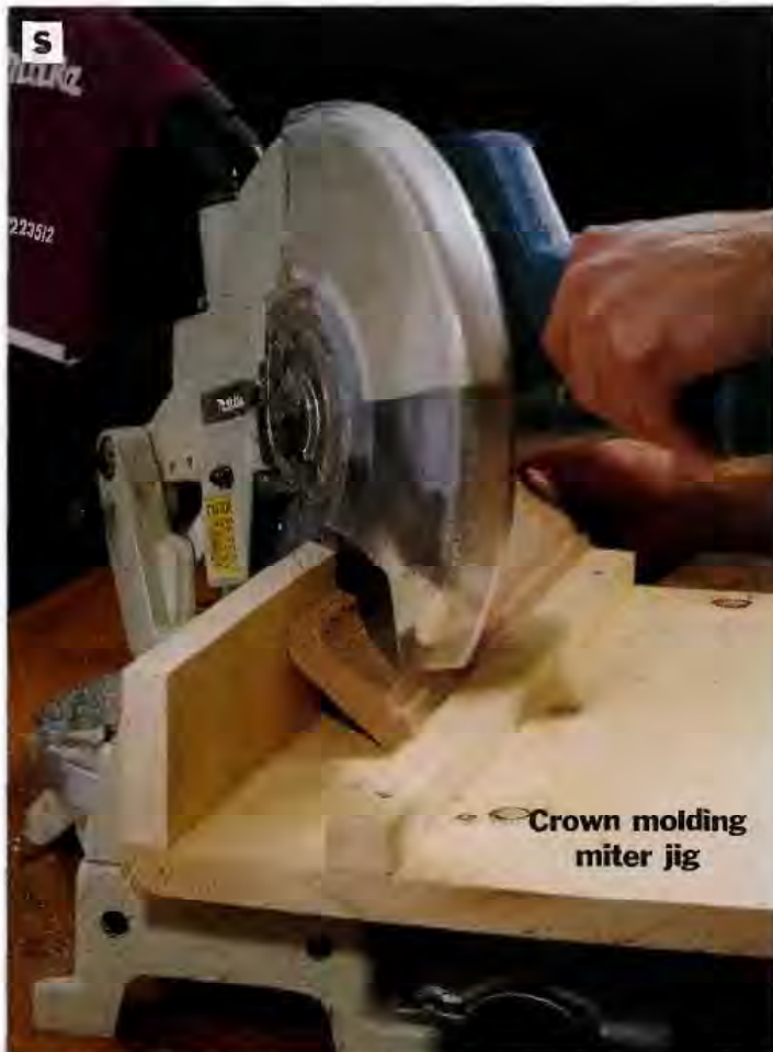
PHOTO S: Miter-cut the ends of the front crown molding strip and the front end of each side strip at 45° to make the crown molding assembly that is attached to the top of the upper cabinet. We used a simple crown molding miter jig to set up the cuts on our power miter saw.
