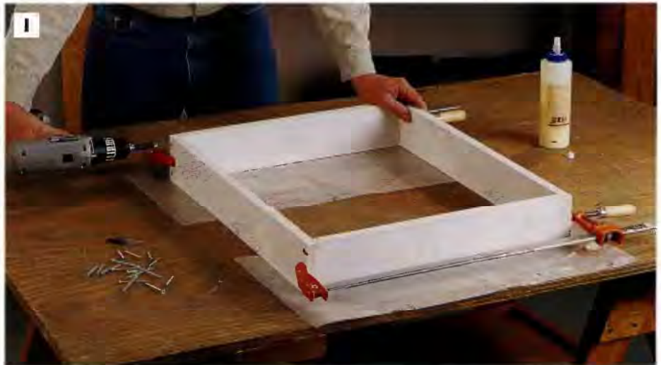
PHOTO I: Glue and screw the drawer ends to the side pieces, driving the screws through countersunk pilot holes to keep the plywood from splitting. Then, fasten the drawer bottom to the bottom edges of this drawer frame. Use the bottom as a guide for squaring up the drawer.
