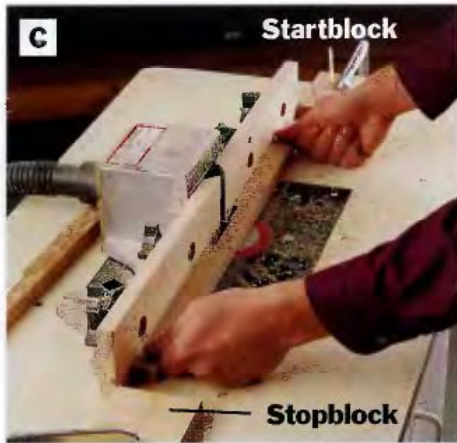
PHOTO C: Make handle cutouts in two back slats using a router table and straight bit. Install start- and stopblocks to limit the length of cut when routing these recesses.
