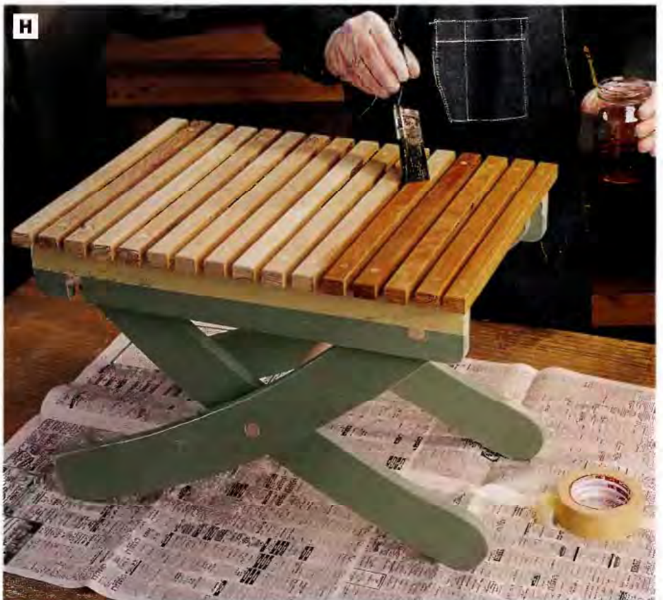
PHOTO H: Coat all raw wood, including the dowels, with Danish oil or another clear exterior-rated wood finish to protect the wood from UV rays and moisture exposure. Use masking tape to keep painted surfaces clean when you brush the slats and dowels with wood finish.
