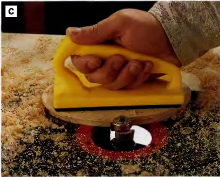
PHOTO C: Use a piloted rabbeting bit in the router table to mill the rabbet around the edges of the lid top. Hold the workpiece securely against the router table and bit with a foam-soled pushpad. Feed the workpiece around the bit clockwise to cut the rabbet.
