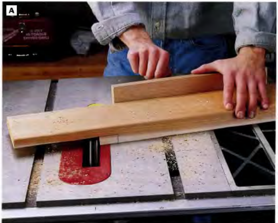
PHOTO A: Cut the half-laps in the seat supports and back supports with a dado-blade set, making multiple overlapping passes. The final pass on each board should be right along the marked cutting line. Set the miter gauge to 65°. Making the half-lap joints prior to cutting the contours of the parts simplifies the layout of the contours.
