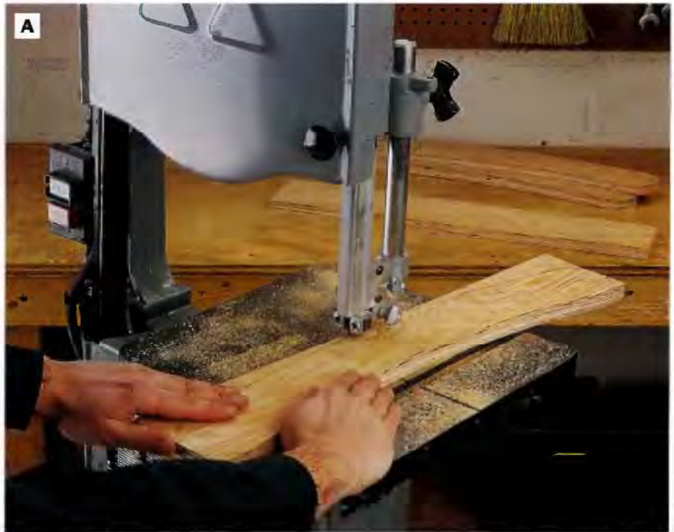
PHOTO A: Lay out and cut the four table legs on the band saw or with a jlg saw. Since the profiles of the legs match, mark and cut one to serve as a template for tracing the profiles onto the other three leg blanks.
