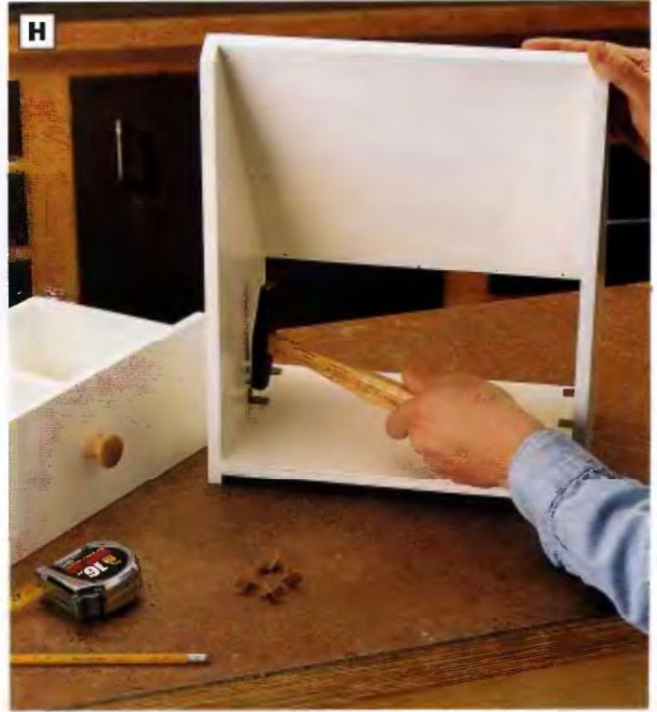
PHOTO H: Tack four nail-on nylon drawer glides to the recipe box bottom inside the drawer opening. The glides should be flush against the project sides.
