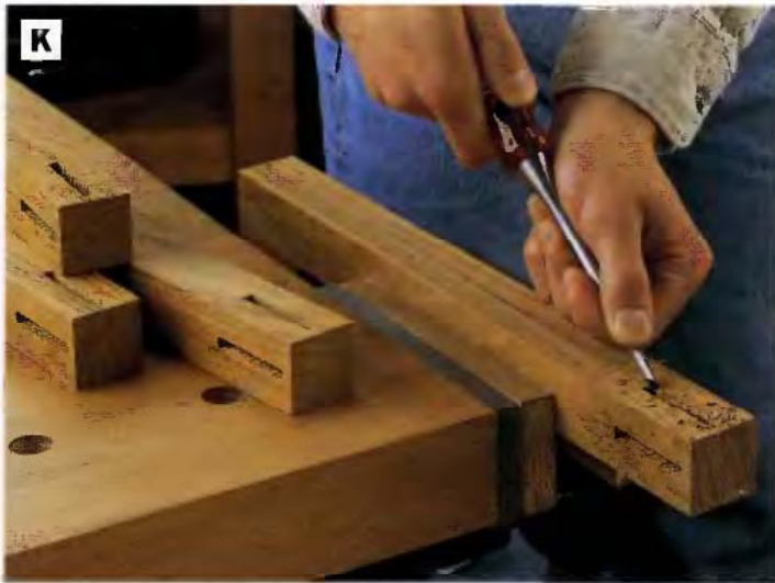
PHOTO K: Drill out the leg mortises on the drill press to ½-in. depth. Clean up the waste from the shoulder of the mortises with a chisel.
