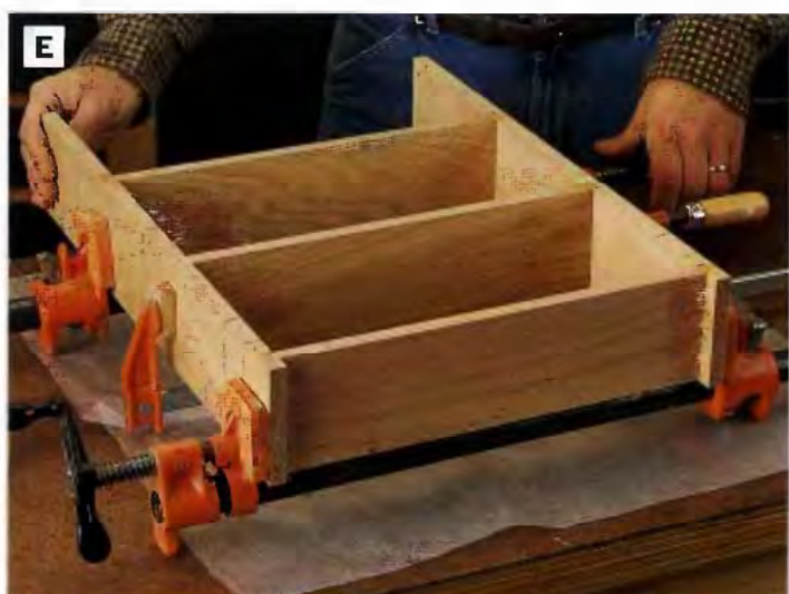
PHOTO E: Spread glue on the mating surfaces of the shelves and sides, and assemble these parts. NOTE: In this photo, the rail notches in the sides are facing down.
