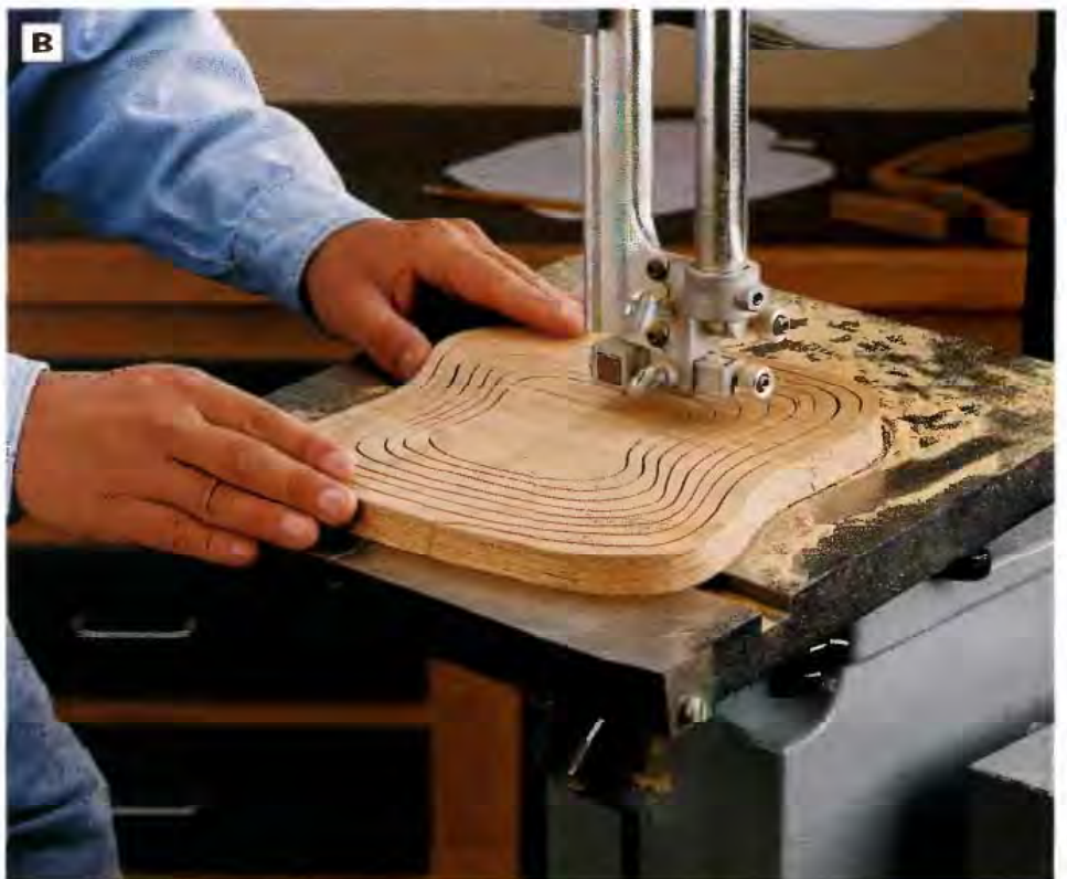
PHOTO B: Tilt the saw table to 3^\circ and begin the spiral cut, orienting the workpiece so the blade tilts in toward the center of the basket throughout the cut. Take your time making this spiraling cut, following your layout lines closely. Try to complete the spirals in one continuous cut.
