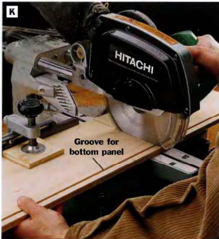
PHOTO K: The sides, front and back for each drawer can be cut from a single 8-ft.-long strip of 1/2-in. plywood. By cutting the groove for the drawer bottom before cross-cutting the parts, you can ensure that the groove will line up on all four parts.
