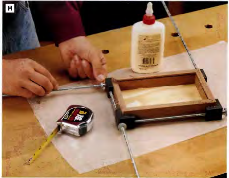
PHOTO H: Glue and clamp the box parts together, with the box bottom in place. We used a frame clamp, which holds all four corners of the box together and squares up the assembly as well. If you use a different clamping method, adjust the clamps until the box is square.
