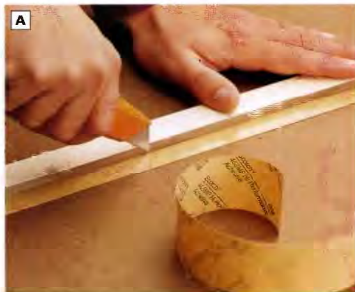
PHOTO A: Peel off the protective paper that covers the adhesive backing of the maple veneer and adhere it to the \frac{1}{4} -in.-thick walnut strips. Trim the veneer to fit the walnut with a sharp utility knife.
