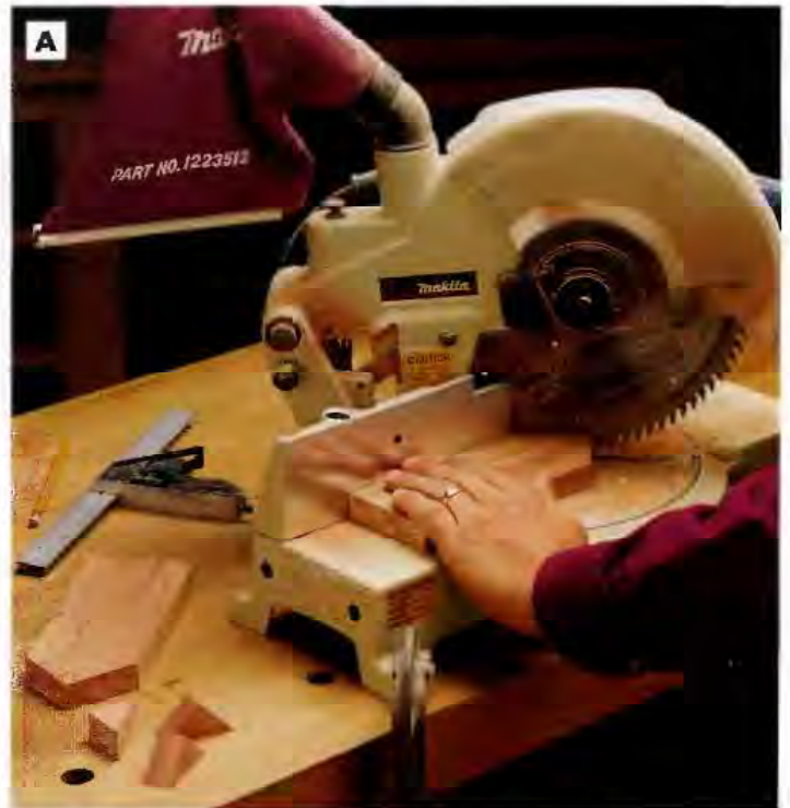
PHOTO A: Trim the gable ends of the sides on a power miter saw with the blade swiveled to 45°. Center the gable peaks across the width of the workpieces.
