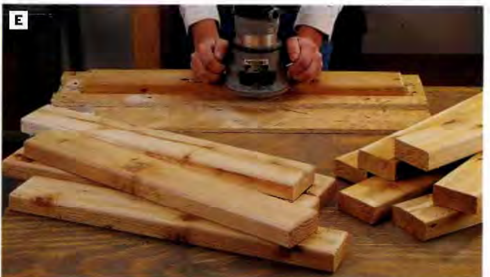
PHOTO E: Cut the 19 seat slats to length, and ease the top edges and ends of each slat with a ½-in. roundover bit in the router. We used a plywood jig clamped to the benchtop to “frame” each slat on all sides and hold it steady while routing. This way, the slats require no further clamping.
