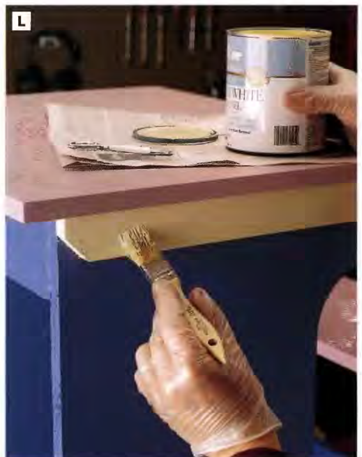
PHOTO L: Conceal the screwheads on the desktop cleats and runners with wood putty and paint.
