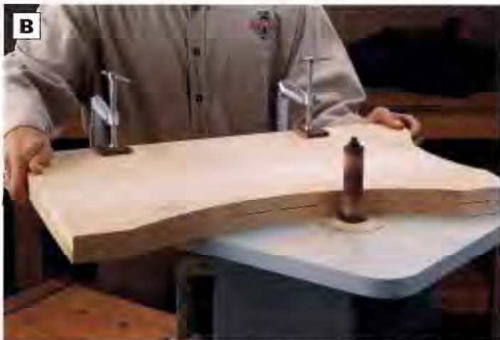
PHOTO B: To smooth the profiles on the sides (and to make them identical), we clamped the sides together and gang-sanded them on an oscillating spindle sander.
