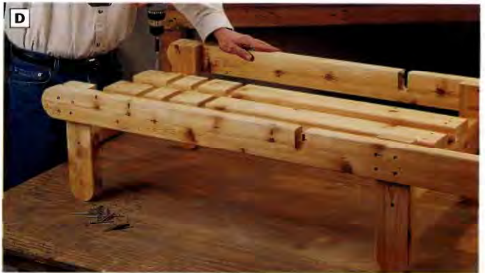
PHOTO D: Fasten the back supports to the seat stretchers. Leave 4½-in. spaces between the back supports and the legs to provide clearance for the chair back rails and adjustment braces.
