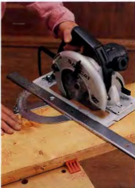
A CIRCULAR SAW and straightedge cutting guide can be used for cross cuts, rip cuts, bevel cuts and miter cuts.
