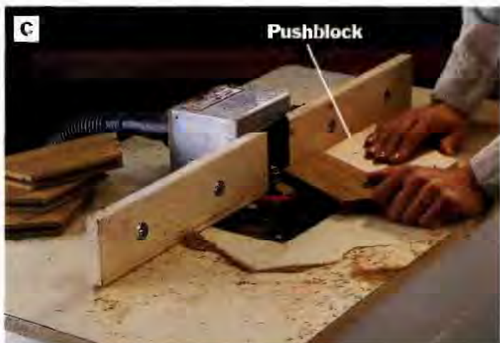
PHOTO C: Rout spline grooves in the angled ends of the tabletop rails. Use a pushblock to aid in running the narrow pieces across the cutter and to back up the cut, preventing chipout.
