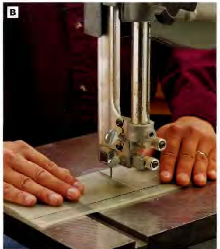
PHOTO B: Measure and cut the Plexiglas end panels on the band saw with a fine-toothed blade. Leave the protective film on the plastic as you machine it, to minimize scratching.
