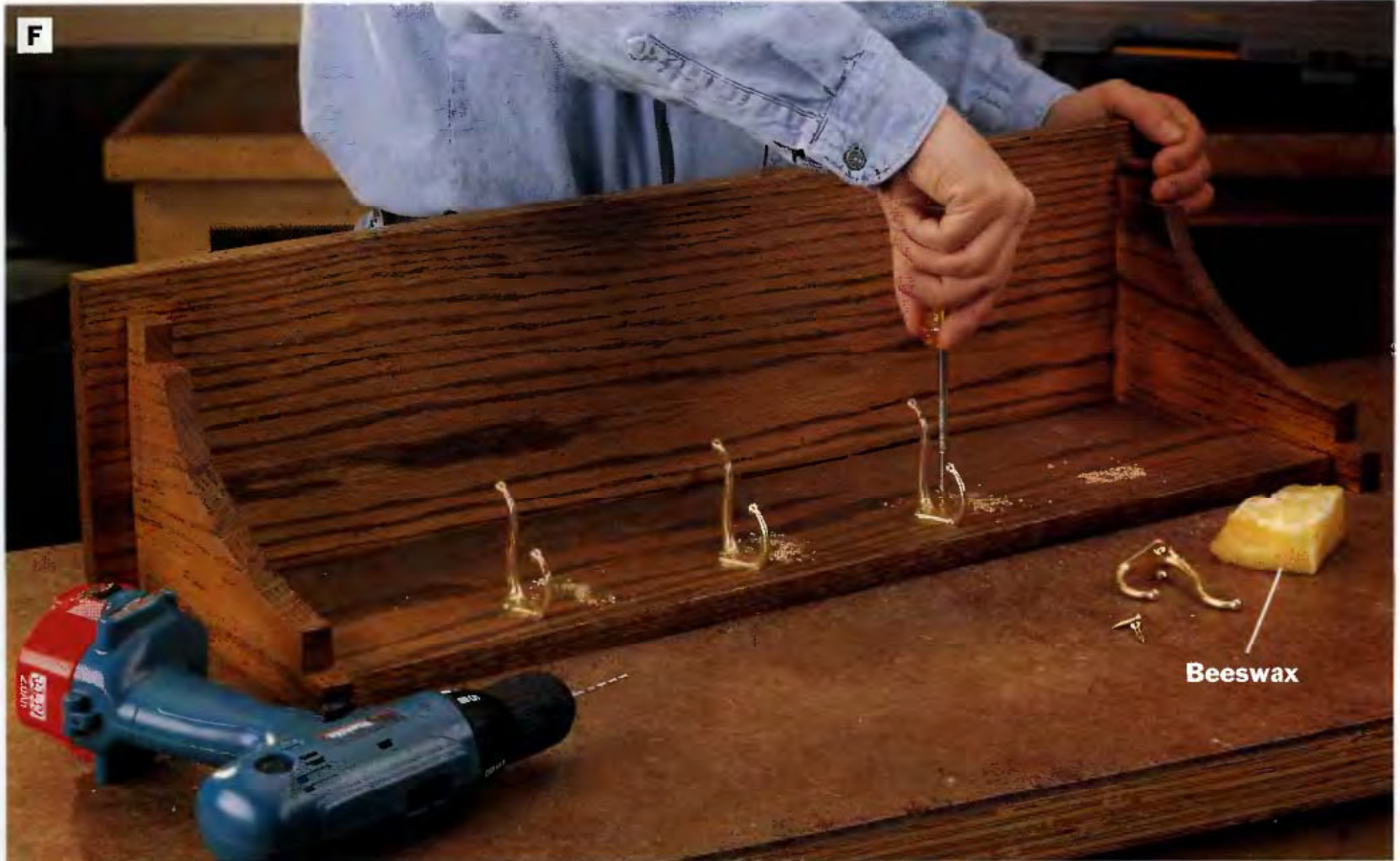
PHOTO F: Lay out and attach four coat hooks to the coatrack back. Drill pilot holes for the screws, especially if the screws are made of brass. Space the hooks about 6 in. apart. Tip: Coat the screw threads with beeswax to make them easier to drive into the oak.
