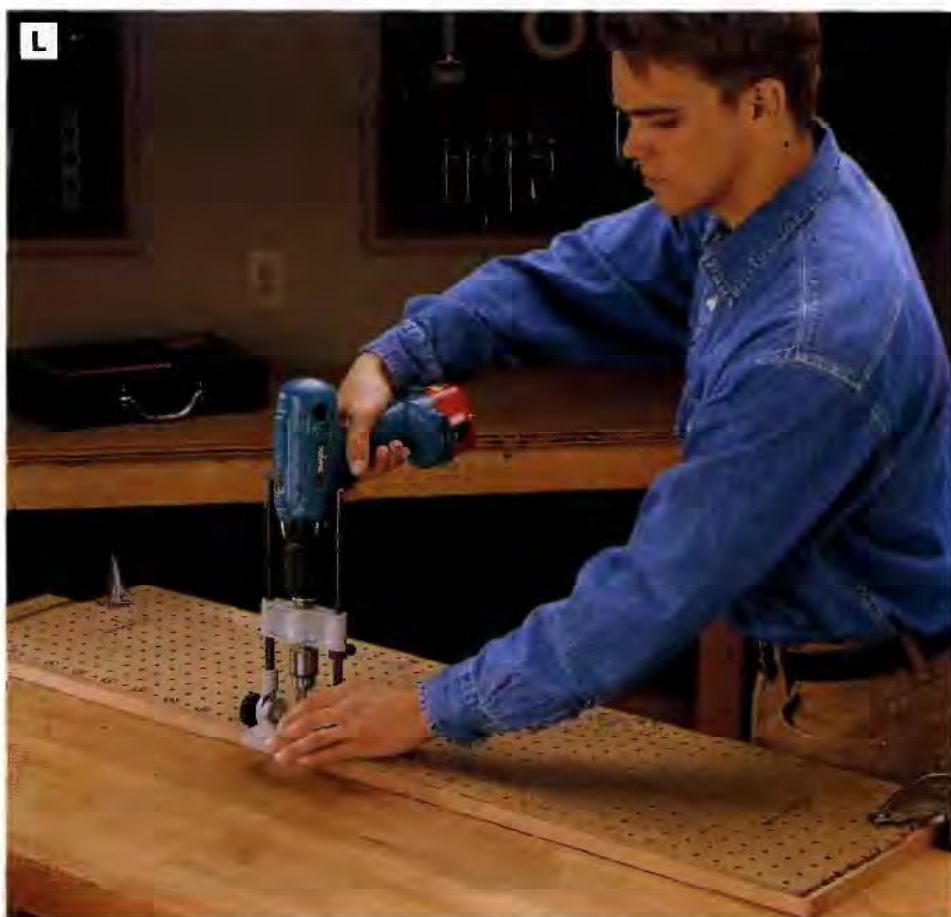
PHOTO L: Drill shelf pin holes in the slide frame stiles using a piece of perforated hardboard as a template and a drill guide to ensure perpendicular holes.
