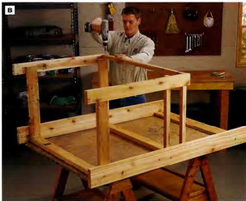
PHOTO B: Assemble the bench framework by attaching the two back stretchers, shelf stretcher and top front stretcher to the end assemblies. The ends of the stretchers should butt against the inside faces of the front and back legs. See Step 4 for exact stretcher placement.
