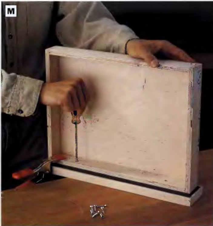
PHOTO M: Clamp the drawer face in position on the drawer front. Drill countersunk pilot holes and drive two 1-in. flathead wood screws to join the parts.
