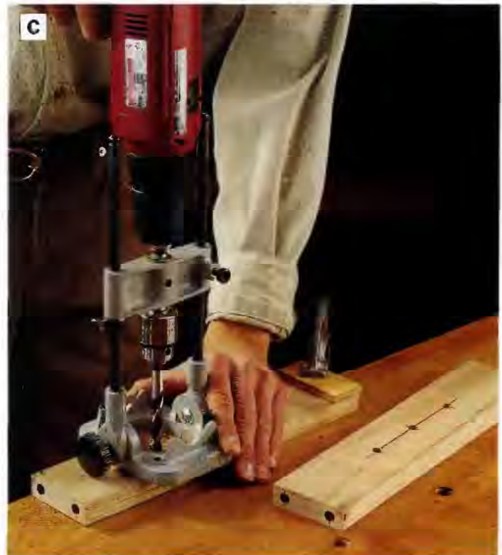
PHOTO C: Drill dowel holes in the bottom shelf rails. We used a portable drill mounted in a portable drill guide equipped with a depth stop. Use a brad-point bit.
