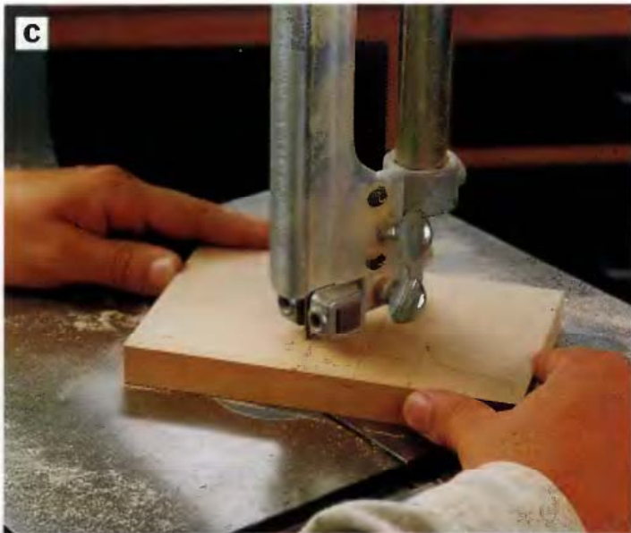
PHOTO C: Lay out and cut one foot to shape on the band saw. Use this workpiece as a template for drawing and cutting the second leg to shape. Then clamp the legs together and sand both smooth at one time.
