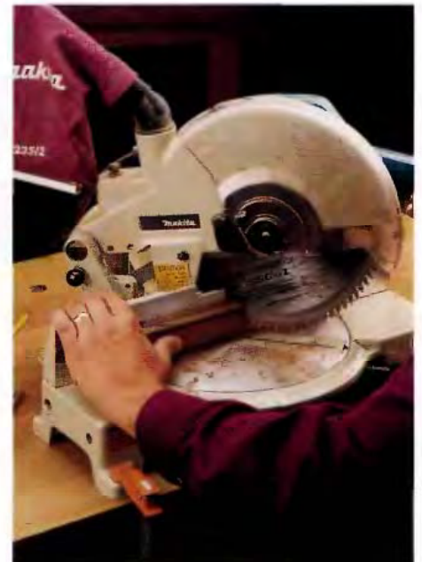
A POWER MITER SAW is perfect for making repetitive cross cuts, including mitered or beveled cuts (bevels require a compound miter saw).
