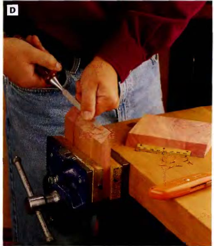
PHOTO D: Mark and cut the shallow hinge mortises into the beveled edges of the roof sections. Score along your mortise layout lines first with a utility knife, then pare out the mortise with a sharp chisel. Keep the mortise depth the same as the hinge leaf thickness.
