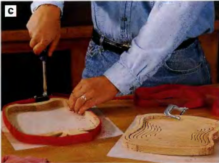
PHOTO C: Glue the saw kerf closed in the frame, and use a strap clamp to hold the joint shut. Glue the first inch or so of the basket spiral together. A C-clamp works well for keeping this joint closed while the glue dries. Then scrape or sand away any glue squeeze-out.
