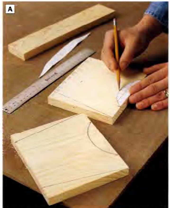
PHOTO A: Draw arched profiles on the stretcher and legs. Full-size paper templates are helpful for drawing these curved shapes.
