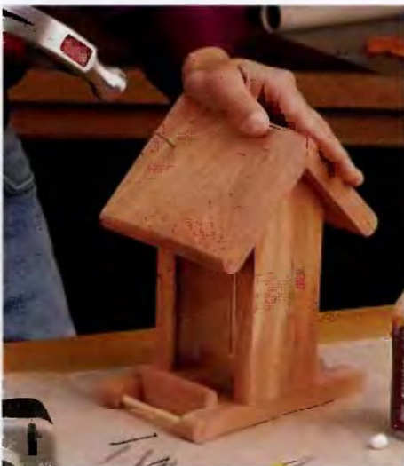
FINISH NAILS are easy fasteners to use for reinforcing butt joints. Drill a pilot hole for each nail before driving it. Set the nail head below the wood surface with a correctly-sized nail set.
