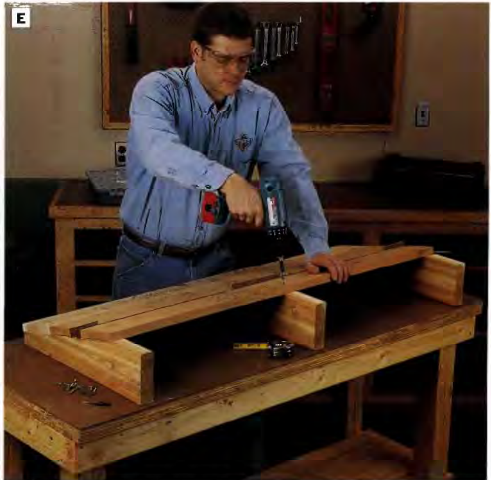
PHOTO E: Attach the back slats along the angled edges of the back supports with screws. Use \frac{1}{4} -in. spacers between the back slats to hold the slats apart.
