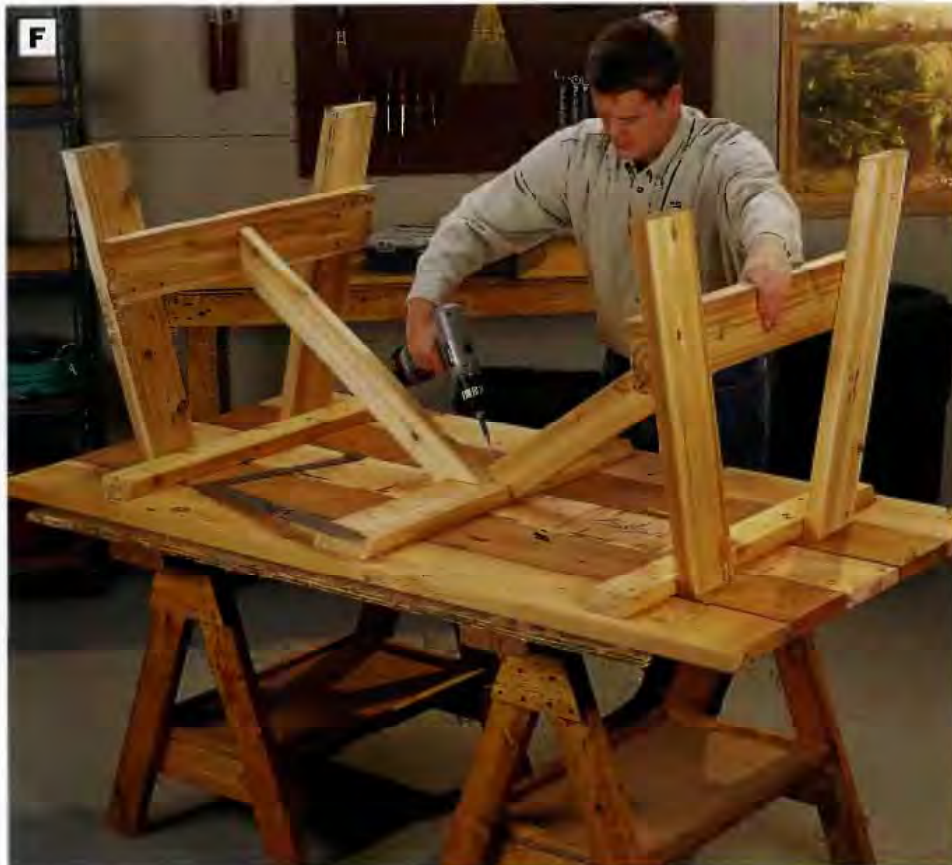
PHOTO F: Fasten the leg assemblies to the outer stretchers, then attach the angled braces to the center stretcher and leg braces. The parts will be easiest to manage if you work with the tabletop turned upside down on sawhorses.
