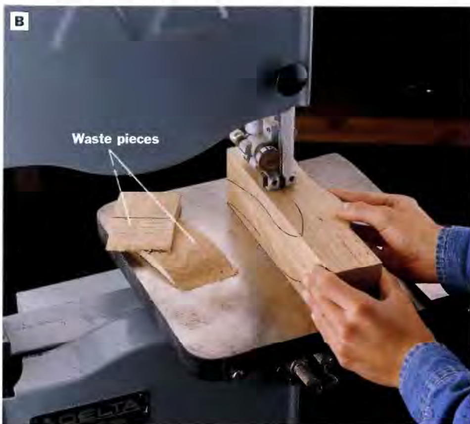
PHOTO B: To cut the legs to shape, start by cutting out the profile on one face of each leg blank on the band saw. Save the waste pieces, and try to cut them out in single sections.
