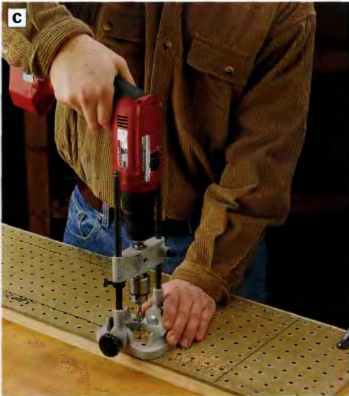
PHOTO C: Drill shelf pin holes in the sides of the upper cabinet, using pegboard as a template. Orient the guide the same way on facing sides to ensure that the holes are aligned.
