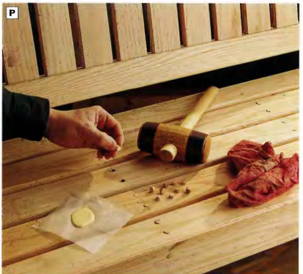
PHOTO P: Conceal all exposed screw heads with oak plugs. You could use oak dowel for making the plugs, but the preferred method is to cut the plugs from the face grain of a piece of oak stock. This way, the plugs will match the wood grain direction of the bench slats.
