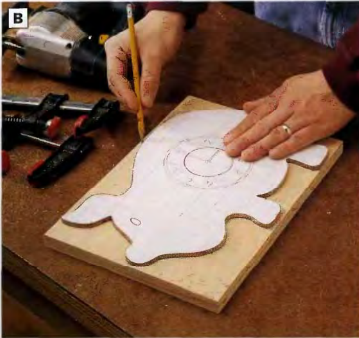
PHOTO B: Trace the template shape onto a piece of plywood, then cut out the clock back with a jig saw.
