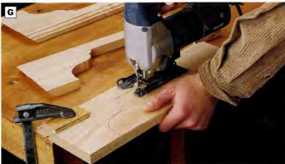
PHOTO G: Cut the pattern shapes in the base trim pieces. We used a jig saw. Wait until you've cut the miters before making the contour cuts so you can be sure each cutout shape is centered and the correct distance from the ends of the trim piece.
