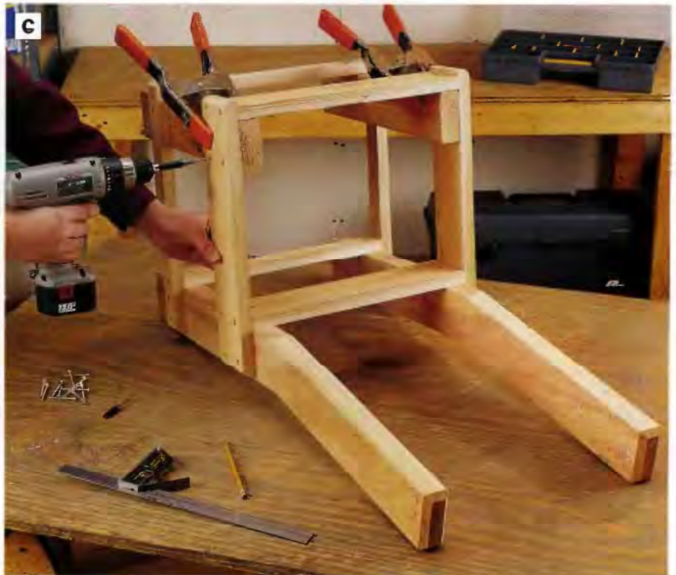
PHOTO C: Attach the upper and lower frames to the back and front legs with countersunk screws.
