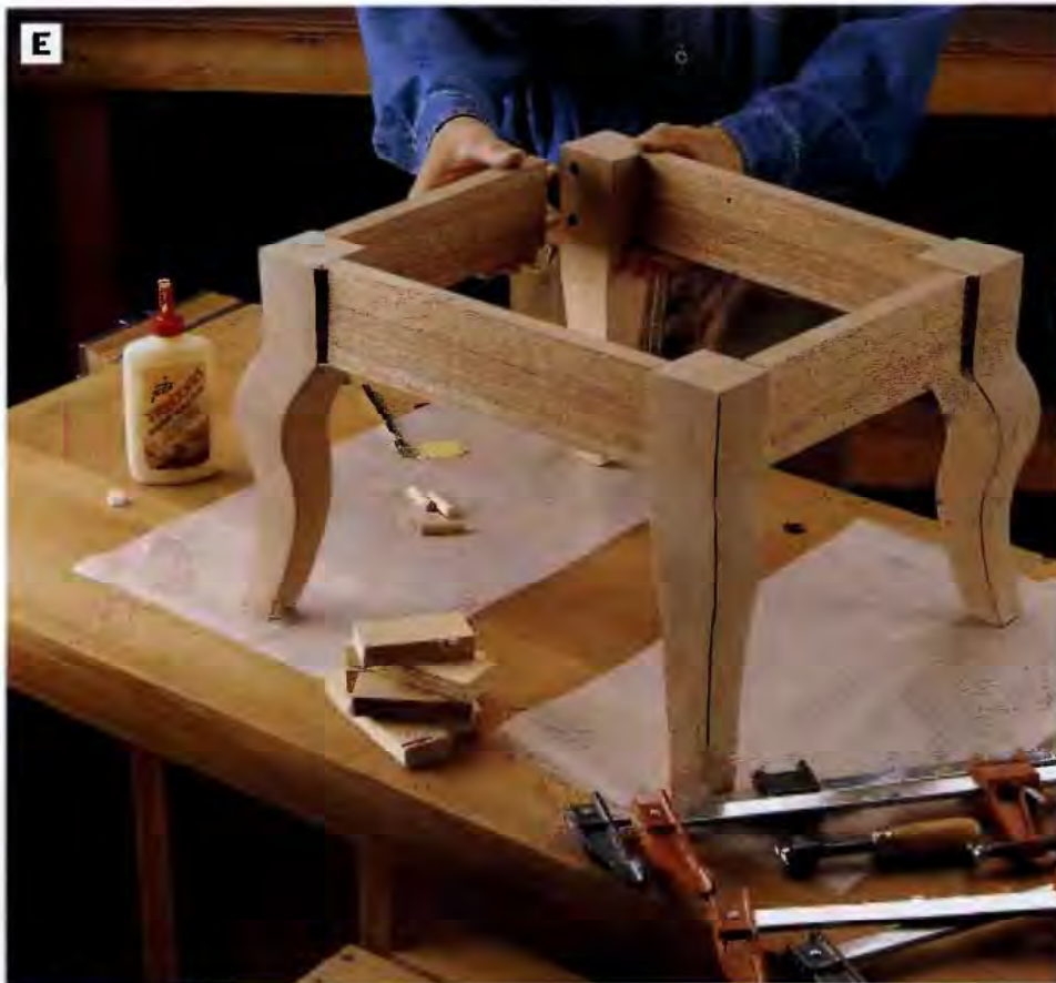
PHOTO E: Glue the dowel joints, insert the dowels and assemble the base. Clamp across the sides with bar or pipe clamps. Measure across the corners of the assembly and square it up.
