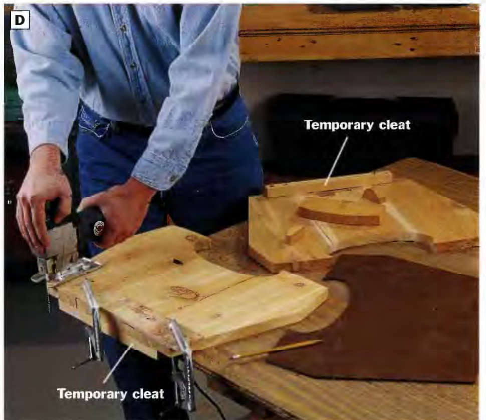
PHOTO D: Assemble two blanks for the deck planter sides using three lengths of 1 \times 8 cedar per blank, fastened together with a temporary cleat. Mark the profiles on the side pieces with a template, then cut the sides to shape. You'll remove the temporary cleats later.
