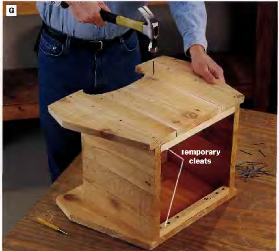
PHOTO G: Fasten the sides to the end/bottom assembly by nailing through the sides and into the ends and bottom. Drill pilot holes before you drive the nails to keep the cedar from splitting. Once both sides are attached, remove the temporary cleats.
