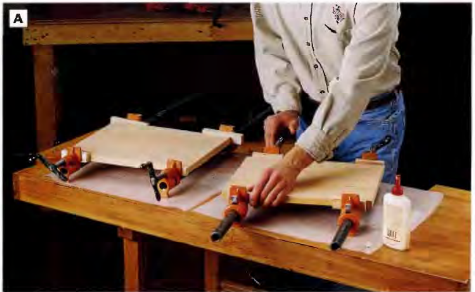
PHOTO A: Edge-glue panels for the sides and the bottom. As you tighten the clamps, the glue will cause the joints to slide out of alignment, so adjust them as well as you can to keep them lined up. Be sure to use clamping pads to protect the wood.
