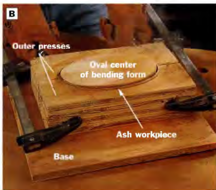
PHOTO B: Steam the ash workpiece until pliable, then remove it quickly from the steamer box and wrap it around the oval center of the bending form. Set the outer presses in place around the ash and clamp the presses together. Tighten the clamps so the ash conforms as closely as possible to the oval center of the bending form. Wear gloves when working with steamed wood—it will be extremely hot.
