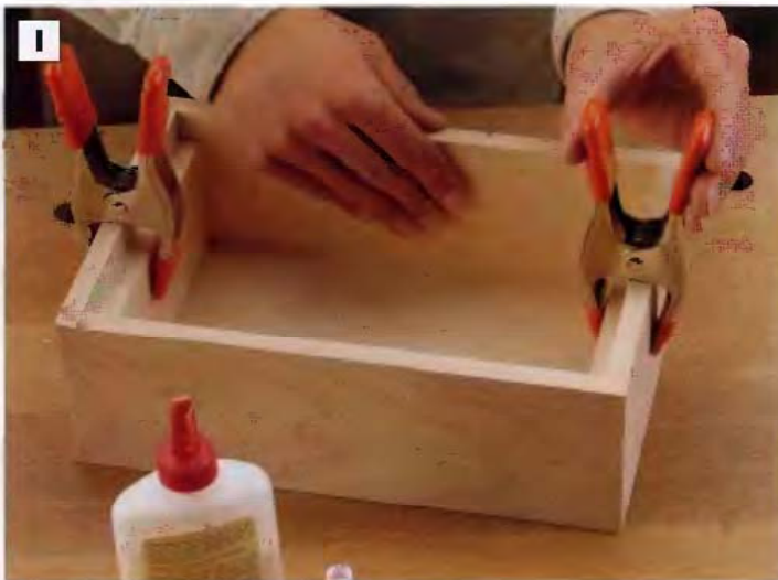
PHOTO I: Glue the tray supports to the inside ends of the box. Butt them against the box bottom and hold them tight with spring clamps.
