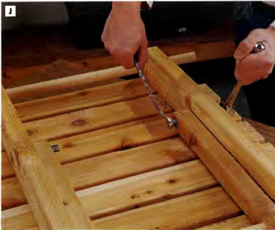
PHOTO J: Install the adjustment brace to the back rest with bolts, washers and nuts. Place a washer on either side of each adjustment brace. Thread two nuts on each bolt and tighten the nuts against one another to lock them together, yet allow the adjustment brace to swing freely.
