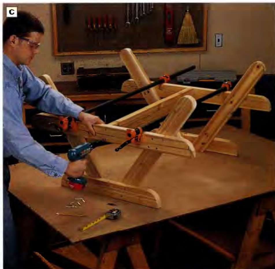
PHOTO C: Stand the leg assemblies top-down to attach the stretcher between them. Hold the stretcher in place with clamps so it is centered on the length of the seat stringers. Drive countersunk 3-in. screws through the seat stringers and into the ends of the stretcher.
