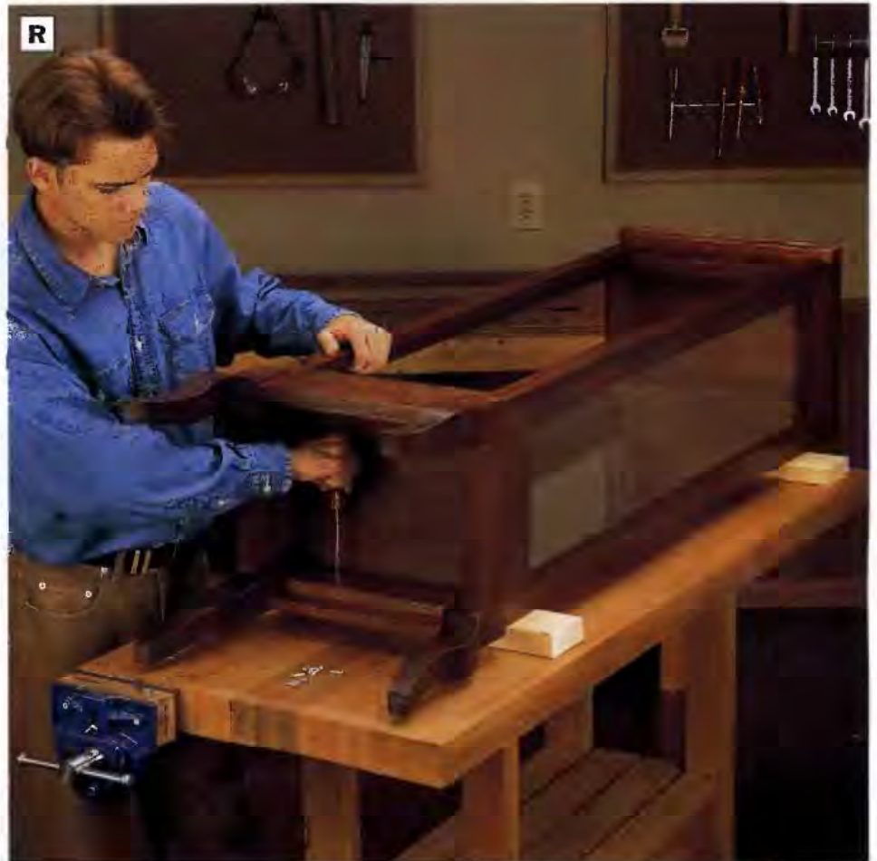
PHOTO R: Attach the base to the cabinet with screws driven through the pilot holes. Set blocks beneath the cabinet to allow clearance for the base.
