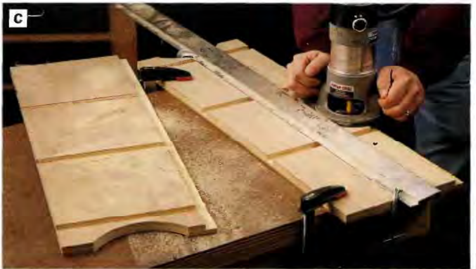
PHOTO C: Rout \frac{3}{4} -in.-wide, \frac{3}{8} -in.-deep rabbets along the inside back edge of each side panel for the bookcase back. Clamp each side panel to your bench to hold it securely as you rout the rabbet, and guide the router base against a straightedge.
