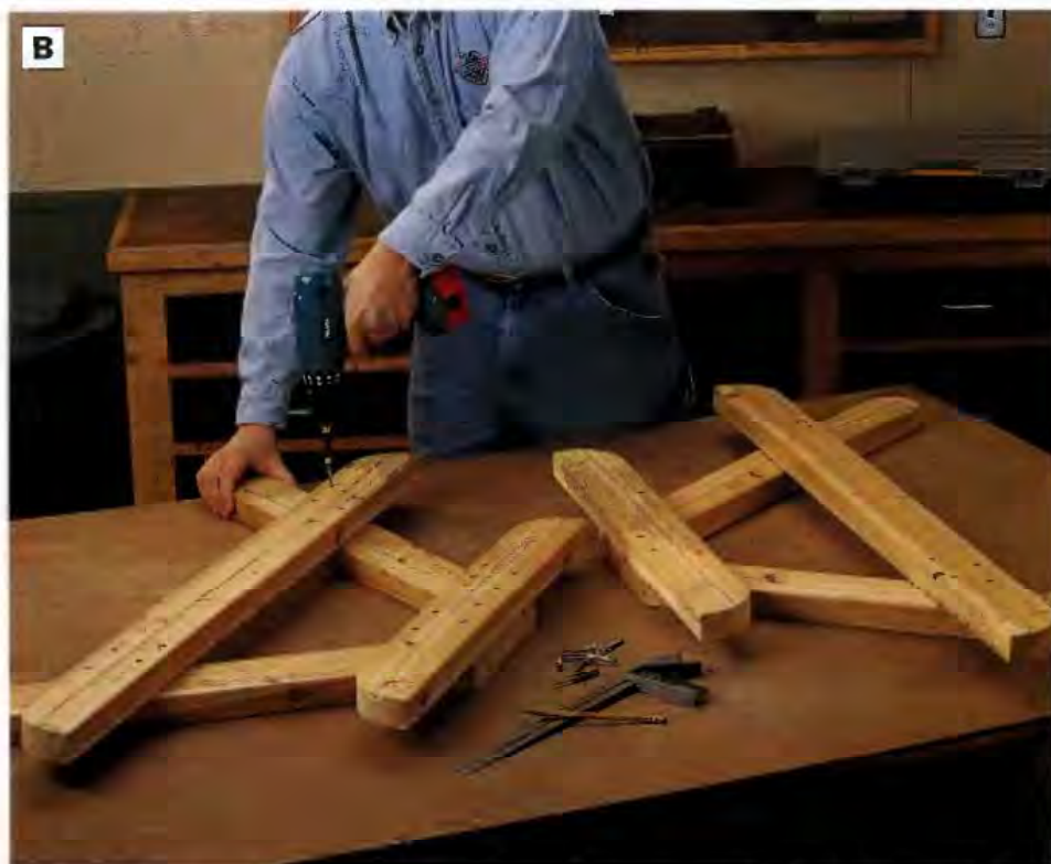
PHOTO B: Set pairs of legs on your worksurface so they splay outward with their angled ends aligned. Attach the top stringers flush to the tops of the legs, and install the seat stringers so they overhang the legs by 8 in. on each end. Fasten the parts with countersunk 2\frac{1}{2} -in. deck screws to form two leg assemblies.
