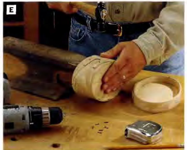
PHOTO E: Drill pilot holes through the fingers on the lid and box sides, then tap the decorative brass pins into the pilot holes and against an anvil to flatten and bend over the pin tips inside the box.
