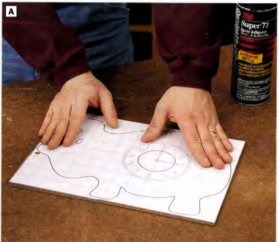
PHOTO A: Enlarge the grid drawing about 400% of its original size to create a full-size paper template for tracing the shape of the clock back. We adhered the paper pattern onto a piece of hardboard to make the template more rigid, then cut out the template shape.
