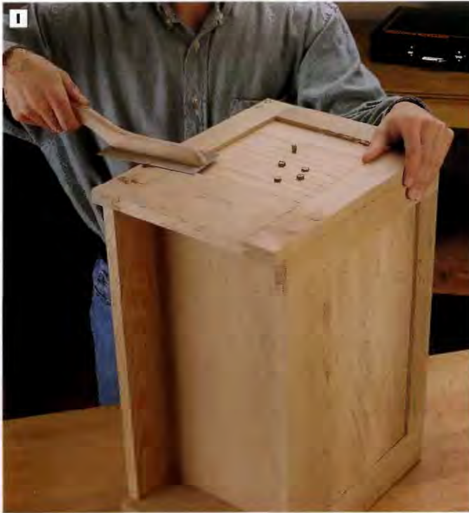
PHOTO I: Use a flush-cutting saw or a dovetail saw to trim the walnut plugs flush. A flush-cutting saw has teeth without set so they won't damage the surrounding wood.
