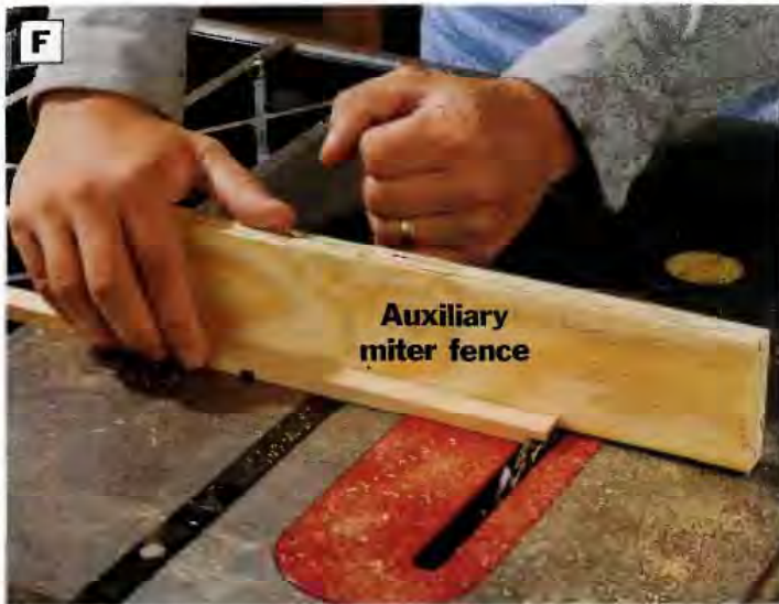
PHOTO F: Cut rabbets and dados into the retainer stiles for the retainer rails. Make these cuts on the table saw with a dado blade, and hold the parts against the miter gauge. We installed an auxiliary fence on the miter gauge to keep the dado blade from tearing out the grain on the retainer stiles.
