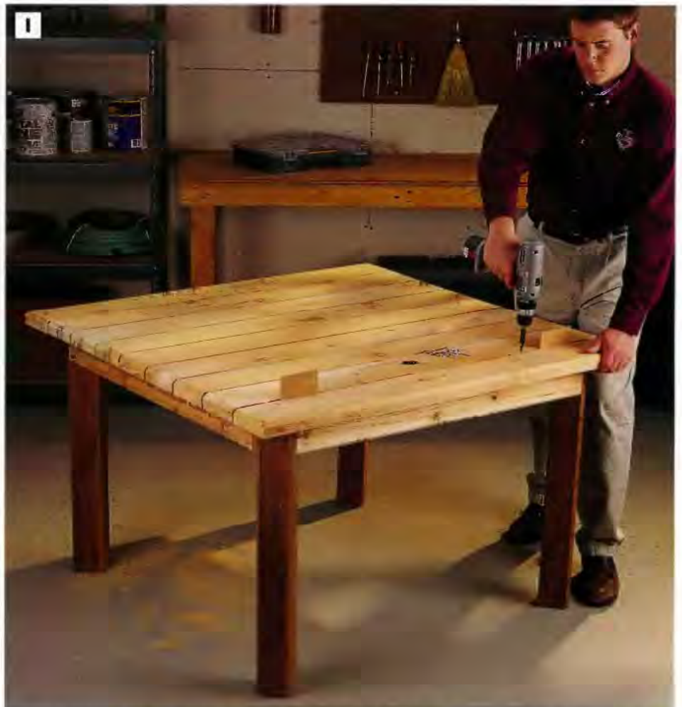
PHOTO I: Attach the top slats to the aprons with 2\frac{1}{2} -in. deck screws. Fasten the center slat first, then work outward. This way, the overhang will be consistent on both ends of the table, and the slats will be evenly positioned. Use a pair of \frac{3}{16} -in. spacers to create uniform gaps between the slats.
