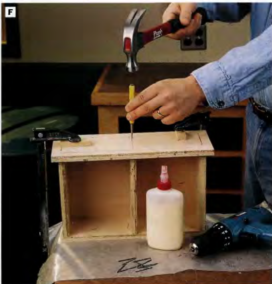
PHOTO F: Install the drawer front on the drawer carcass with glue and finish nails. Note that the front overhangs the drawer carcass \frac{5}{8} in. on the sides and \frac{1}{2} in. on the top and bottom.
