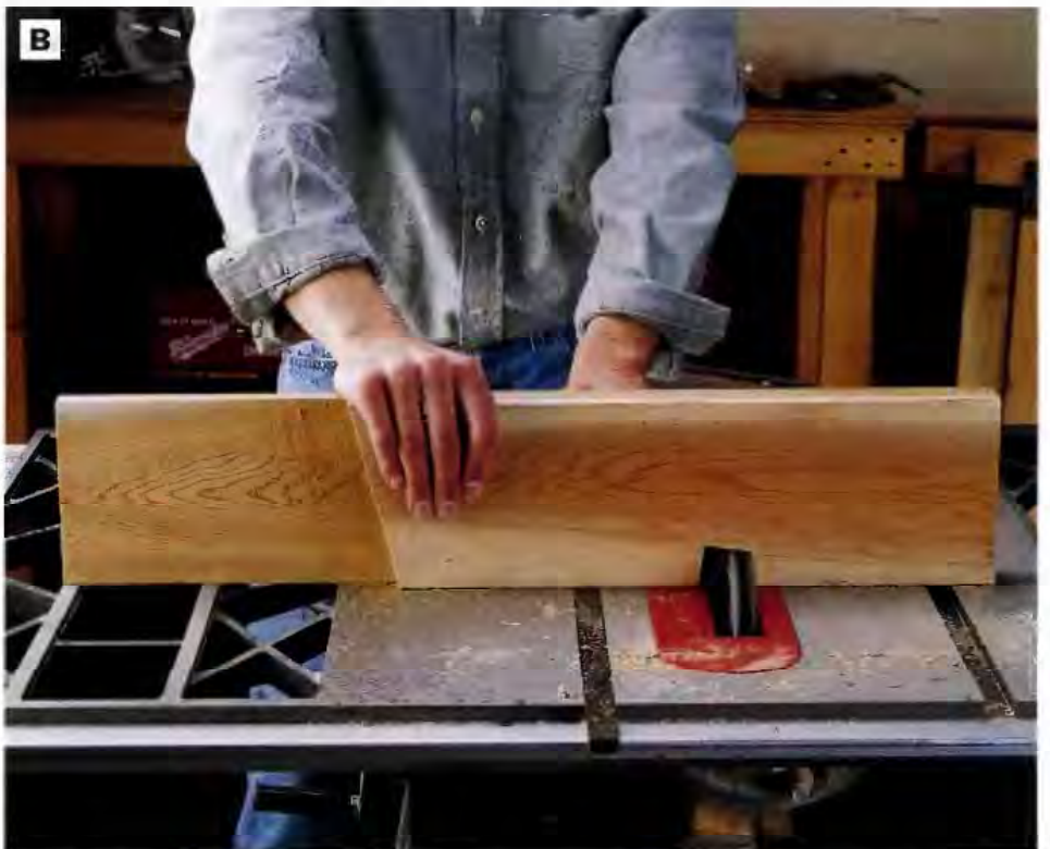
PHOTO B: Set the cutting angle of the dado-blade set to 7° and cut 1-in.-deep notches for the seat supports into the bottom edges of the seat supports.
