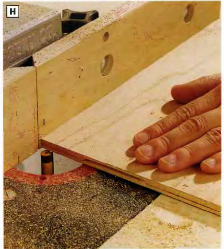
PHOTO H: Rout a shallow rabbet around the top face of the bottom panel for the veneer inlay strips. Install a 1/2-in. straight bit in your router table to cut this 1/2-in.-deep rabbet. Practice on scraps first and test the fit of the strips in the rabbet.
