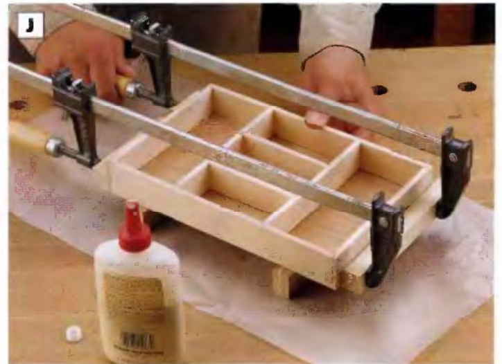
PHOTO J: After the tray dividers are assembled, glue up the tray sides and ends and tack the tray bottom in place with brads.
