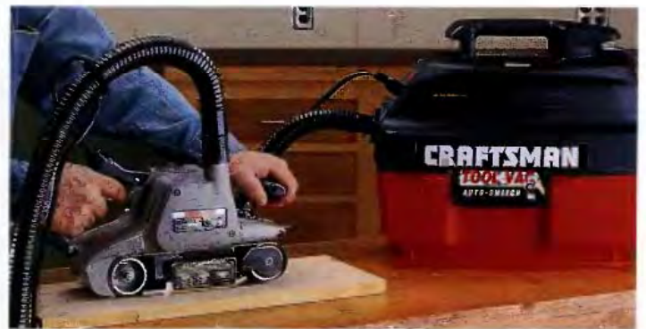
A TOOL VAC is a relatively new entry in the dust collection field. It's similar to a shop vac in size and power. Tools are connected to the power source through a receptacle mounted on the tool vac. This allows the vac to shut on and off automatically as the tool is used.
