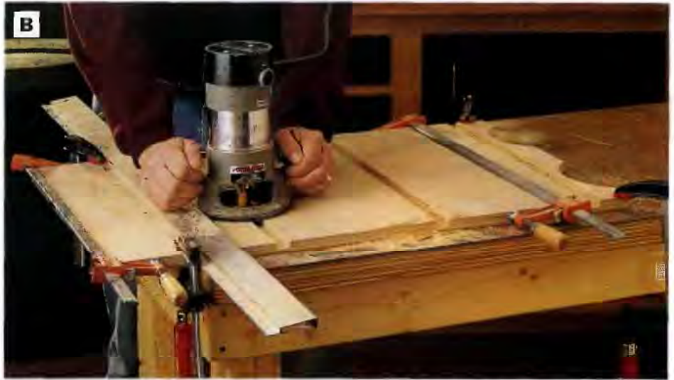
PHOTO B: Clamp the sides together side by side, lay out the shelf dado locations and gang-rout the dados across both sides. Clamp a straightedge across the side workpieces to guide the router cuts.
