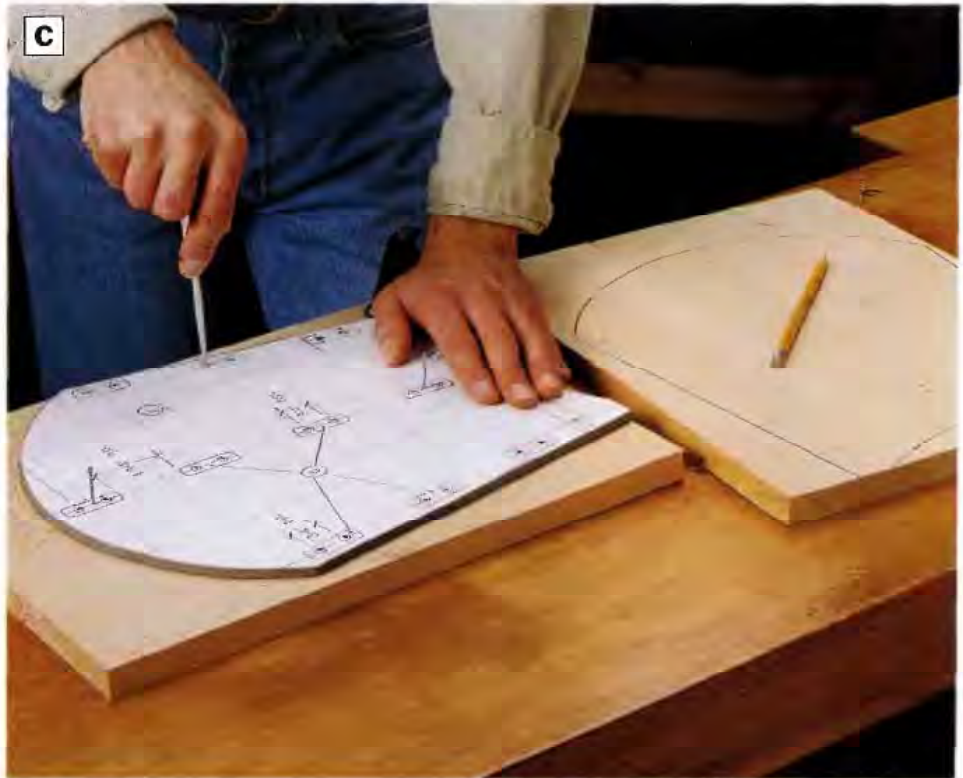
PHOTO C: Center the template on each side panel and outline the shape. Poke an awl or centerpunch through the template holes to mark centerpoints for the dowel holes.
