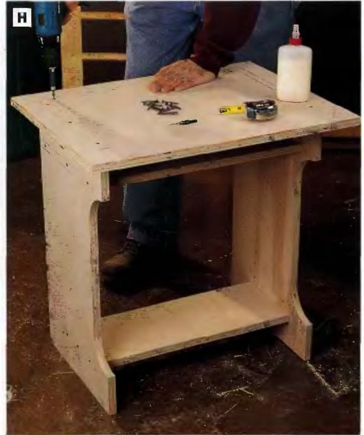
PHOTO H: install the desktop on the legs and shelf back with glue and countersunk 2-in. drywall screws. Mark the positions of the legs and shelf back on the desktop for locating the screws.
