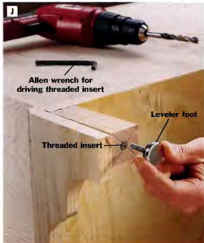
PHOTO J: Leveler feet are attached to the foot blocks to protect the floor and to allow you to adjust the height of the cabinet to conform to unevenness in the floor.
