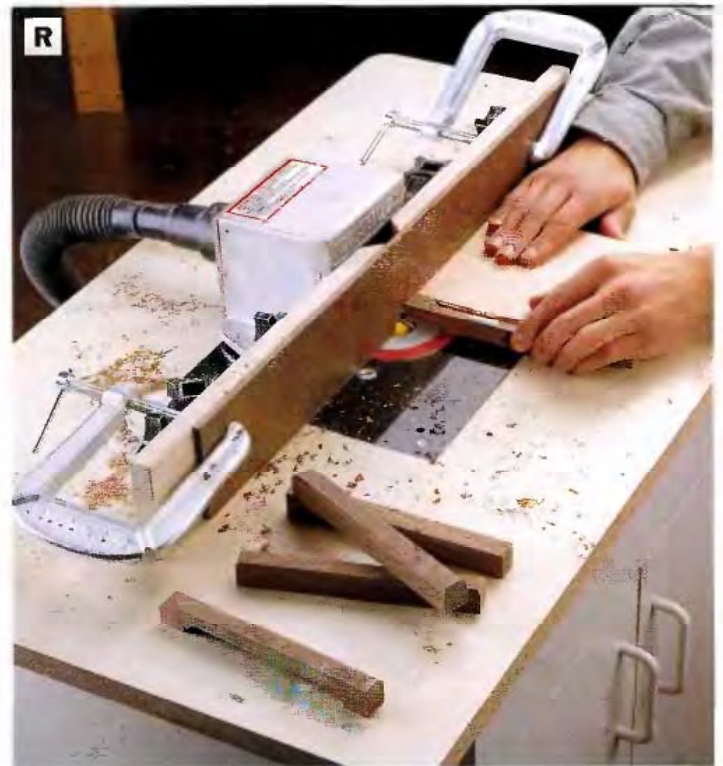
PHOTO R: Rout chamfers on the long edges of the handles first. Then use a backup pushblock to cut the chamfers into the ends of the handles (on the front faces of the handles only).
