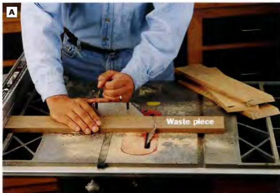
PHOTO A: Crosscut the front, back and side pieces to length on the table saw with the blade tilted to 45°. Since all four parts are the same length, you can use the saw fence as an index to establish the length of the parts, like we show here. CAUTION: If you use this method, the blade must tilt away from the fence, and the waste piece must fall away on the side of the blade opposite the fence. Otherwise, the waste piece or the workpiece could become trapped between the blade and the fence and result in kickback.
